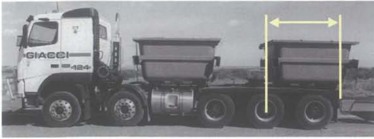
Fig. 3(b) Side view of rigid truck (hauling unit) showing the coupling rear overhang dimension.
