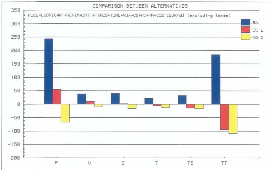
Figure 10 – Total costs at production cost price by vehicle categories at different junction types vs intersection
