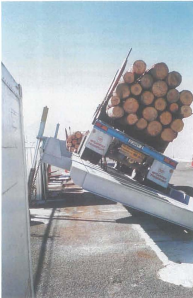
Figure 3 - Tilt table test on a 4-axle log trailer.
