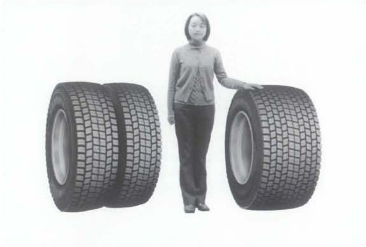
Figure 1 – The super-single drive (GMD) tyre, right, and the conventional dual tyres.
