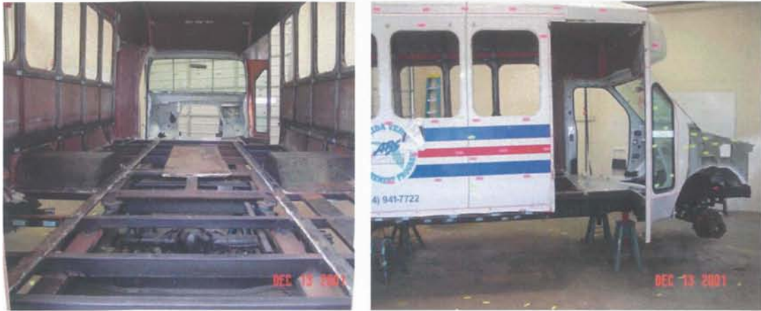
Figure 8. Disassembled Ford Eldorado Aerotech 240 transit bus.
