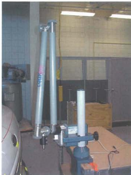
Figure 1 – Portable digitizing device: FARO Arm
