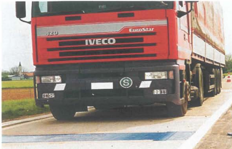
Figure 3 – Reference and Enforcement Scale.- Designed as Dynamic Axle Weighbridge
