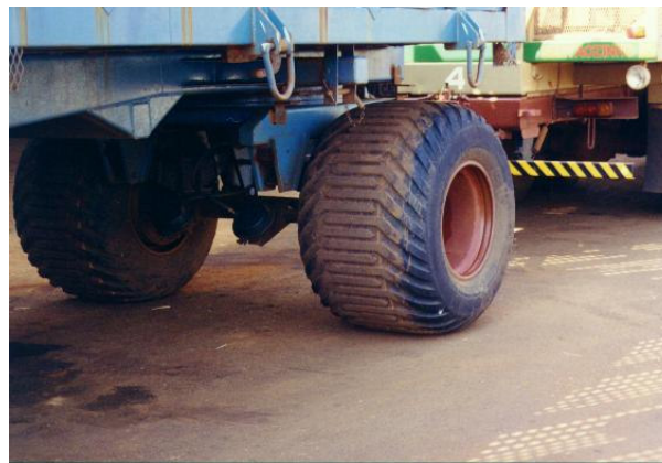
Figure 6. Trelleborg tire in a rear single axle (70 cm wide).
