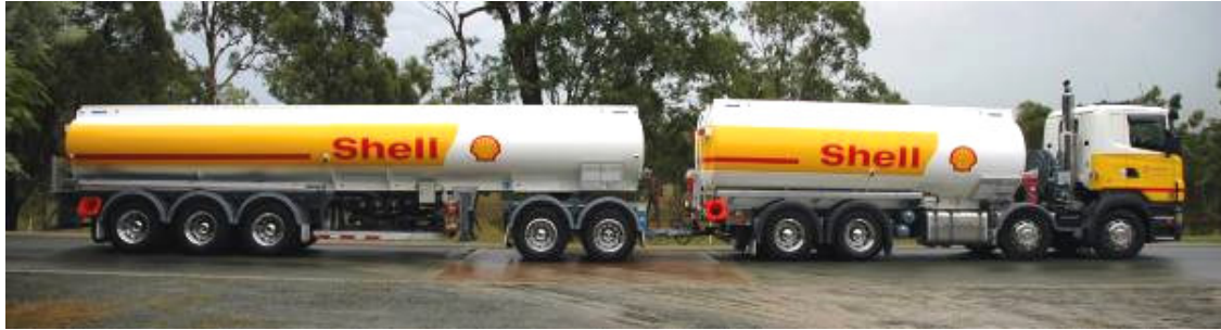
Figure 2. PBS vehicle–SD2255–22 meters (72 feet), 55 tonnes (121,000 pounds)
