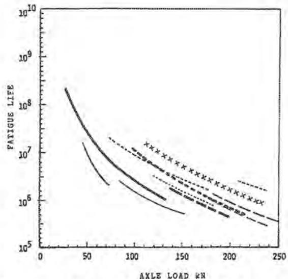
The comparisons of different axles based on the horizontal strains in the asphalt concrete
