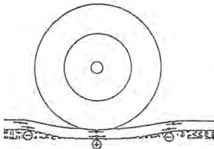
Compressive (-) and tensile (+) stresses under a wheel load. Deformations not to a scale
