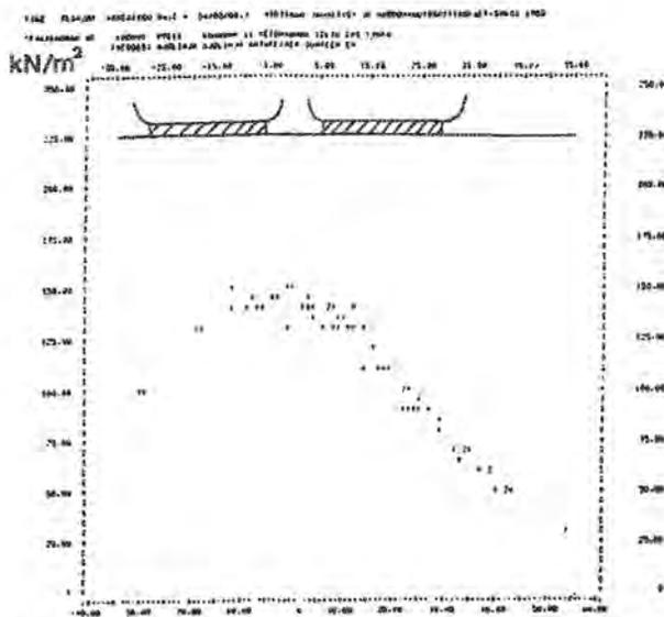
An example of stresses depending on the transversal position of a wheel
