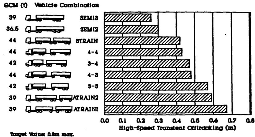
Figure 6. High-Speed Transient Offtracking results
