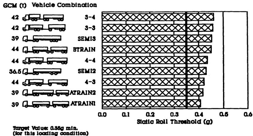
Figure 4. Static Roll Threshold results, typical NZ vehicles
