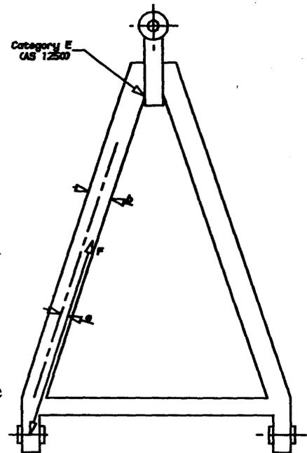
$$\begin{aligned} \text{Axial Stress } \sigma_a &= F/A \\ \text{Bending Stress } \sigma_b &= F \cdot e \cdot y/I \\ \text{If } e \approx 1/3 b & \quad \sigma_a = \sigma_b \end{aligned}$$
