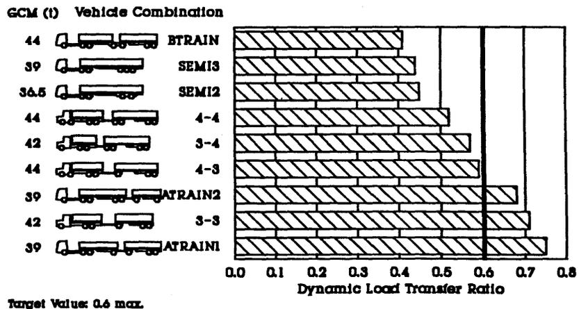
Figure 5. Dynamic Load Transfer Ratio results
