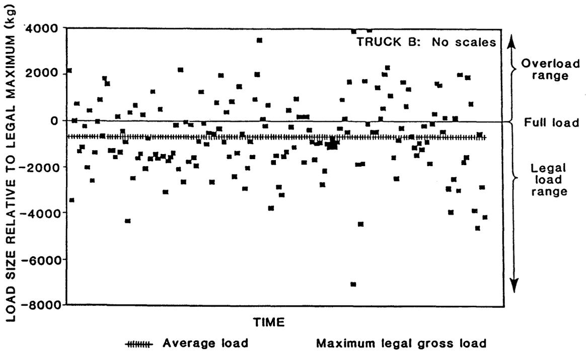
Figure 4. Payload Distribution for a Truck without a Scale System.
