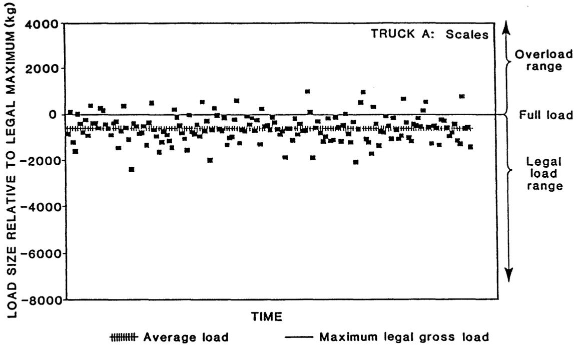
Figure 3. Payload Distribution for a Truck with a Load-Cell System.
