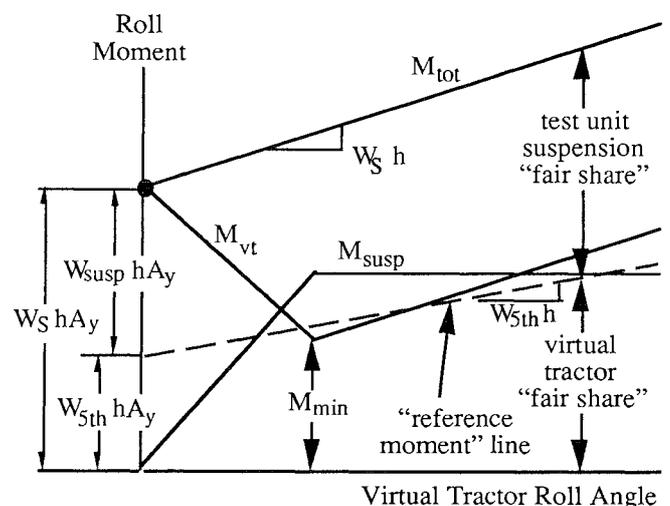
Figure 3. Mechanics of the payload unit tilt table test
