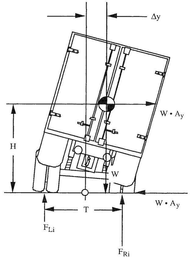
Figure 1. A heavy truck in a steady turn
