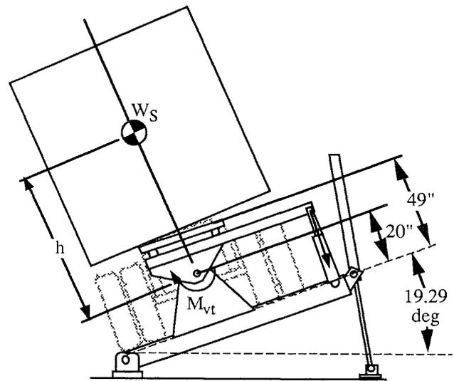
Figure 2. A tilt test using the virtual trailer
