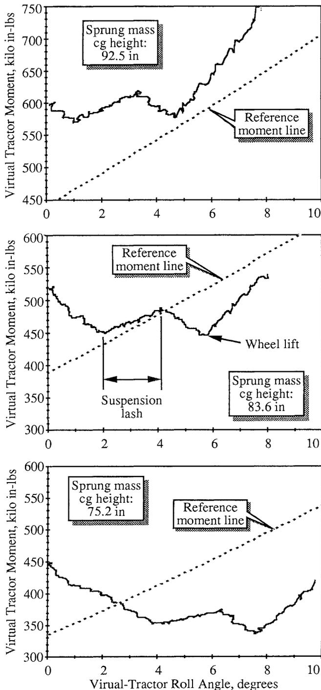
Figure 8. Tilt-table data from tests of a semitrailer with three different cg heights
