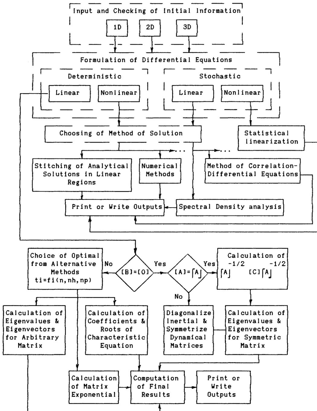
Fig. 2. Simplified functional scheme of IMITA (1D, 2D and 3D - chain, planar and spatial structure; [A], [B] and [C] - inertial, damping and stiffness matrices of linear system;  $t_i$  - simulation time necessary for  $i$ -th method,  $f_i$  - simple algebraic functions,  $n$  - simulated system degrees-of-freedom,  $n_h$  and  $n_p$  - parameters characterizing the complexity of excitations and outputs; [ ] and [ ] denotes arbitrary and symmetric matrices)
