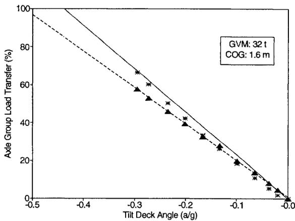
Fig. B3 - Roll-threshold calibration for the IPEC pantechnicon.
