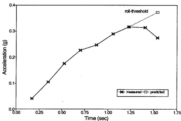
Fig. 4 - Method of predicting the time to the roll-threshold.
