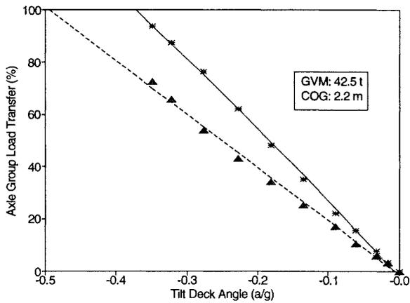
Fig. B1 - Roll-threshold calibration for the SHELL fuel tanker.
