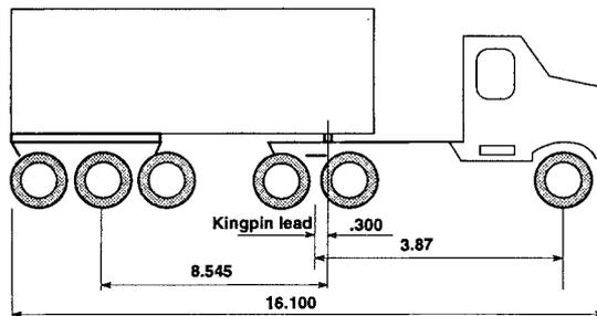
Fig. A5 - Vehicle dimensions for the Linfox flour tanker .
