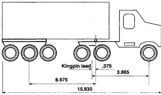
Fig. A1 - Vehicle dimensions for the Shell fuel tanker.
