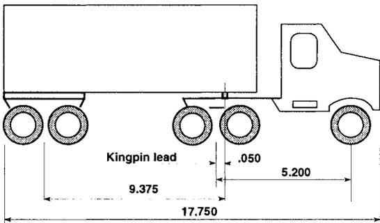
Fig. A3 - Vehicle dimensions for the IPEC pantechnicon.
