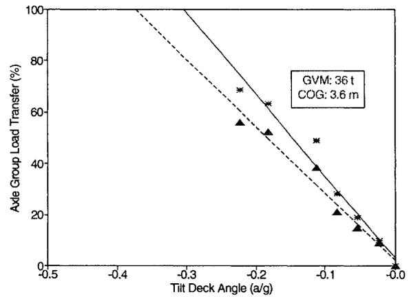
Fig. B2 - Roll-threshold calibration for the V/Line flatbed trailer (Wool).
