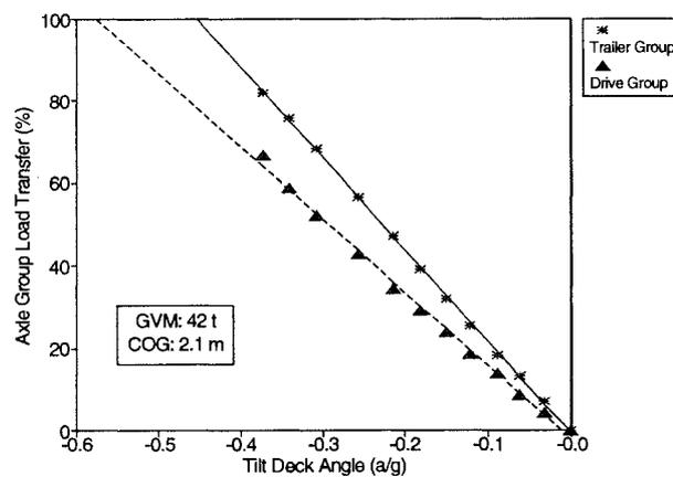
Fig. B5 - Roll-threshold calibration for the Linfox flour tanker.
