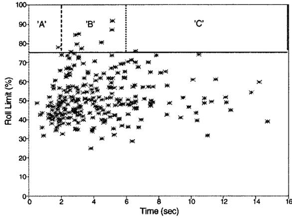
Fig. 3 - Critical recorded times to reach maximum lateral acceleration from zero or steady state acceleration.
