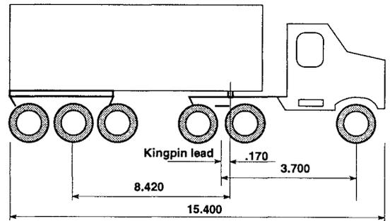
Fig. A4 - Vehicle dimensions for the Linfox fuel tanker.
