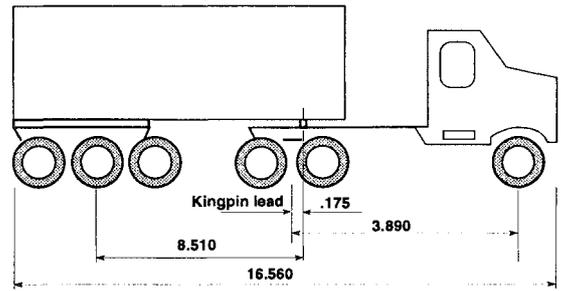
Fig. A2 - Vehicle dimensions for the V/Line flatbed trailer (Wool).
