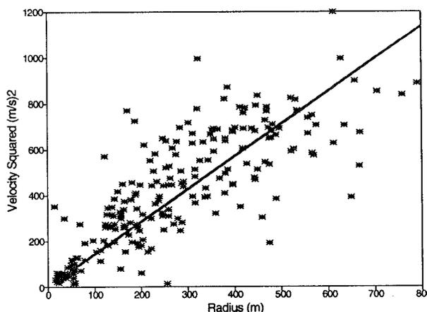
Fig. 2 - Drivers' preferred choice of vehicle speed and steer path.
