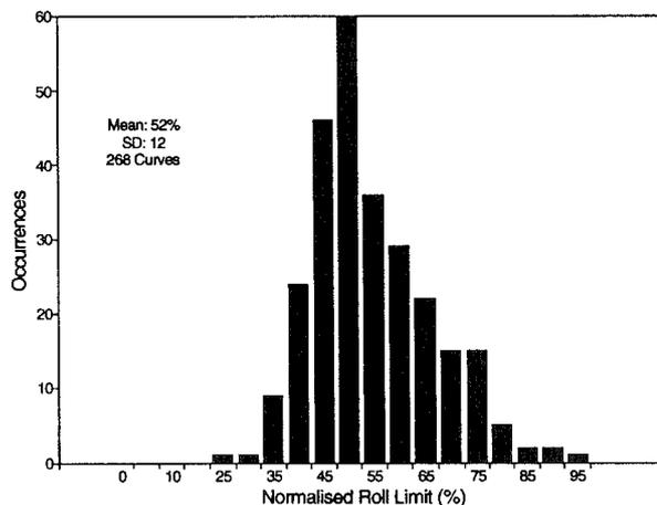
Fig. 1 - Test vehicles distribution to the roll-limit.
