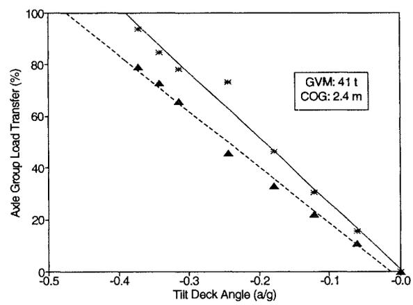
Fig. B4 - Roll-threshold calibration for the Linfox fuel tanker.
