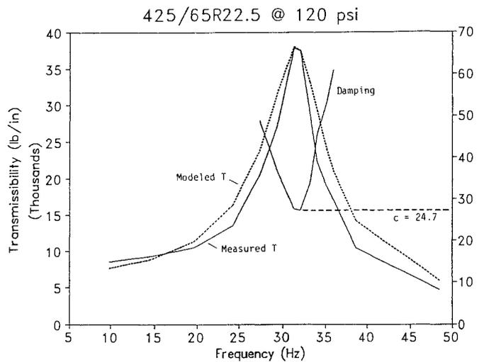
Fig. 12. Comparison of transmissibility predicted by the tire model with measured transmissibility. Damping coefficient,  $c$ , as a function of frequency.
