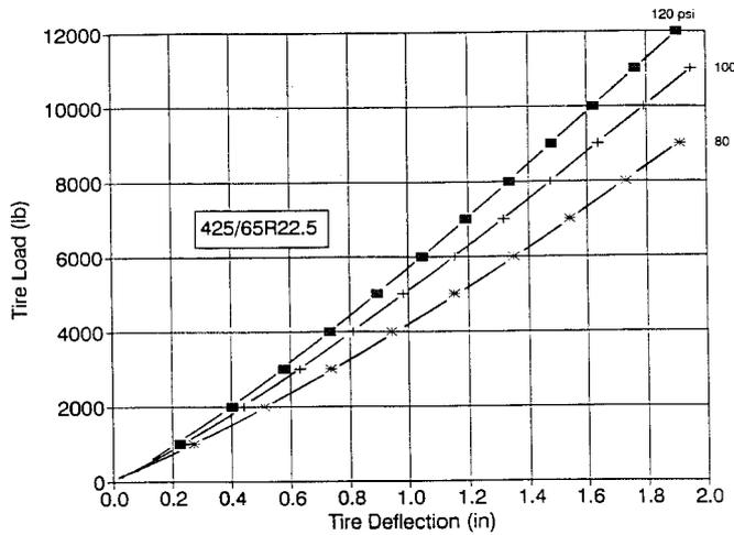
Fig. 4. Load vs. deflection - wide base tire
