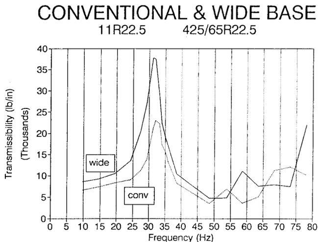
Fig. 10. Comparison of transmissibility data measured for the conventional and the wide base tire
