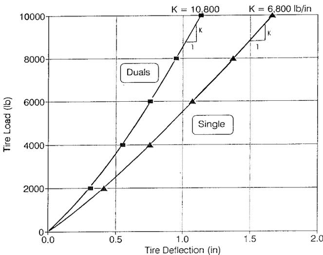
Fig. 5. Comparison of load-deflection data for dual tires and a single wide base tire
