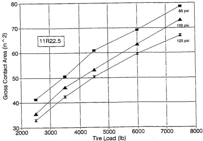
Fig. 7. Effect of tire load on footprint area of the conventional truck tire
