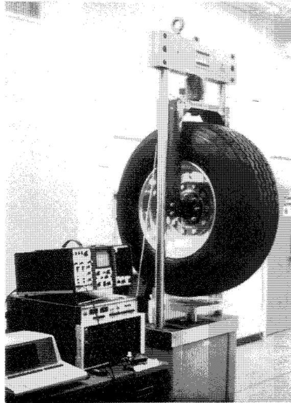
Fig. 2. Wide base tire mounted in the MTS testing machine
