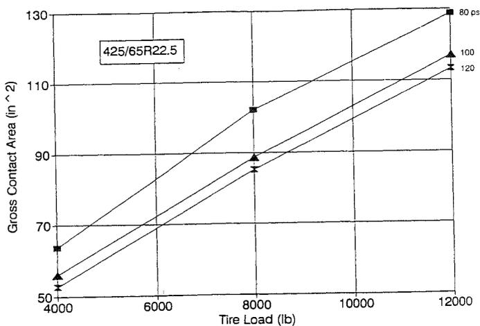
Fig. 8. Effect of tire load on footprint area of the wide base truck tire
