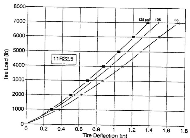
Fig. 3. Load vs. deflection, conventional tire
