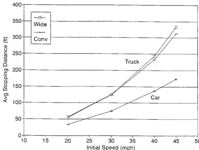
Fig. 18. Comparison of tractor/trailer and passenger car stopping distances
