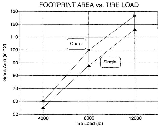
Fig. 9. Comparison of the footprint area of dual tires and a wide base single tire at the same inflation pressure
