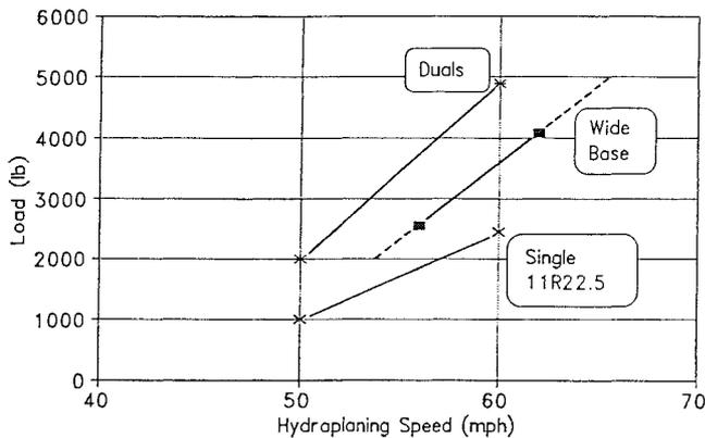
Fig. 20. Effect of load on hydroplaning speed
