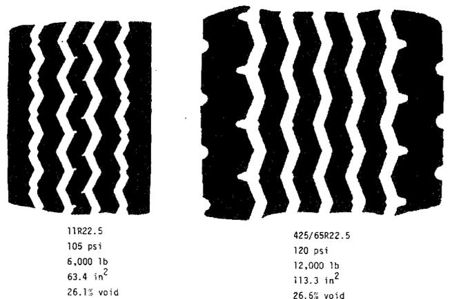
Fig. 6. Video image footprints of a conventional and a wide base tire
