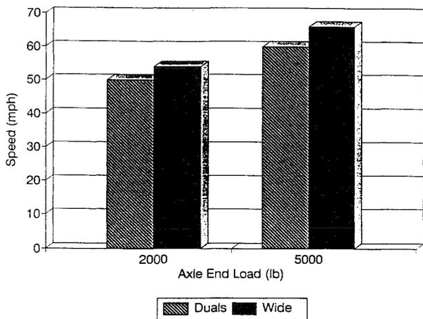
Fig. 21. Hydroplaning speed comparison
