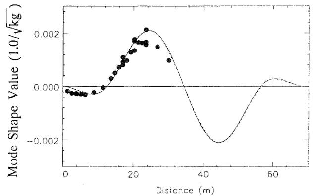
Fig. 3. First flexural mode of the Drift Road bridge. Measured ● Theory —
