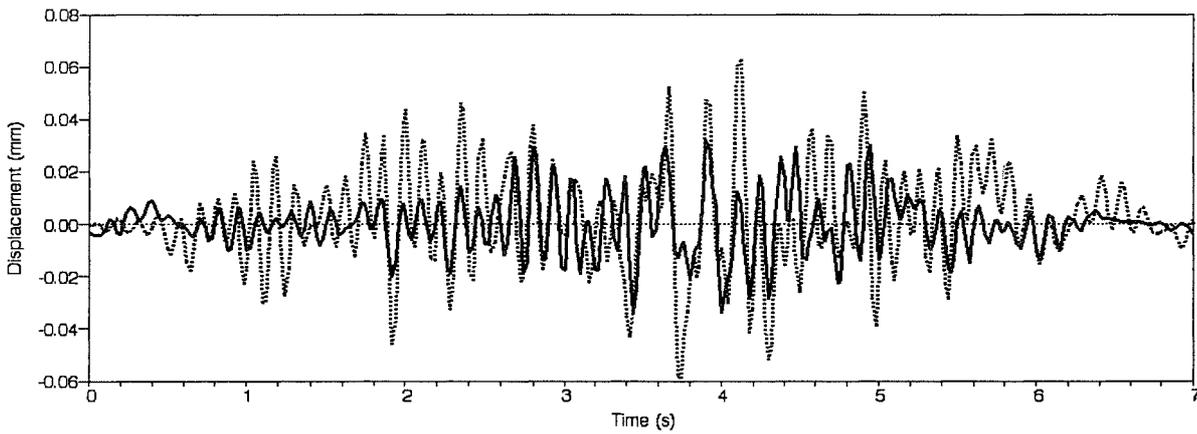
Fig. 9. Validation results for the Drift Road bridge. Bridge responses measured at midspan. Vehicle travelling south-east to north-west at 50 km/h. Measured ——— Predicted - - - - -
