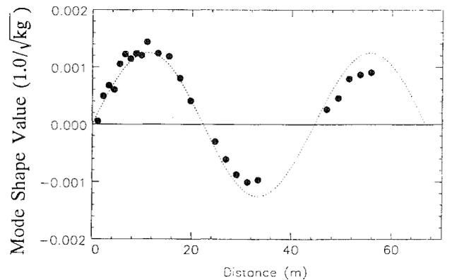
Fig. 4. First flexural mode of the Lower Earley bridge. Measured ● Theory - - -
