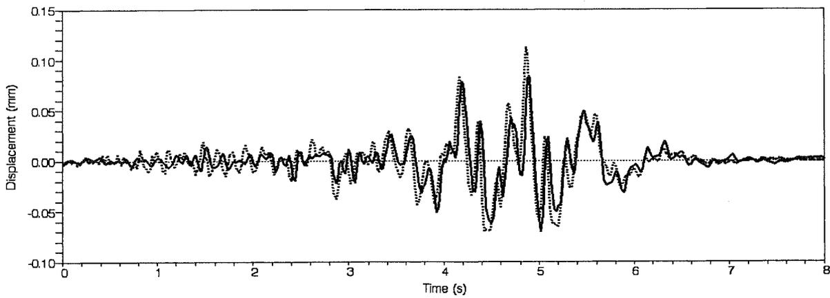
Fig. 10. Validation results for the Lower Earley bridge. Bridge responses measured at midspan. Vehicle travelling south to north at 50 km/h. Measured ——— Predicted - - - - -
