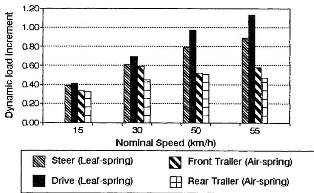
Fig. 7. Maximum dynamic load increments for the Drift Road bridge.
