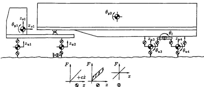
Fig. 11. 11 degree of freedom, 2 dimensional tractor and trailer vehicle model with leaf-spring suspensions (After Cole (ref. 5))
