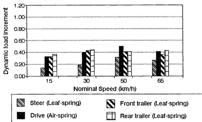
Fig. 8. Maximum dynamic load increments for the Lower Earley bridge.
