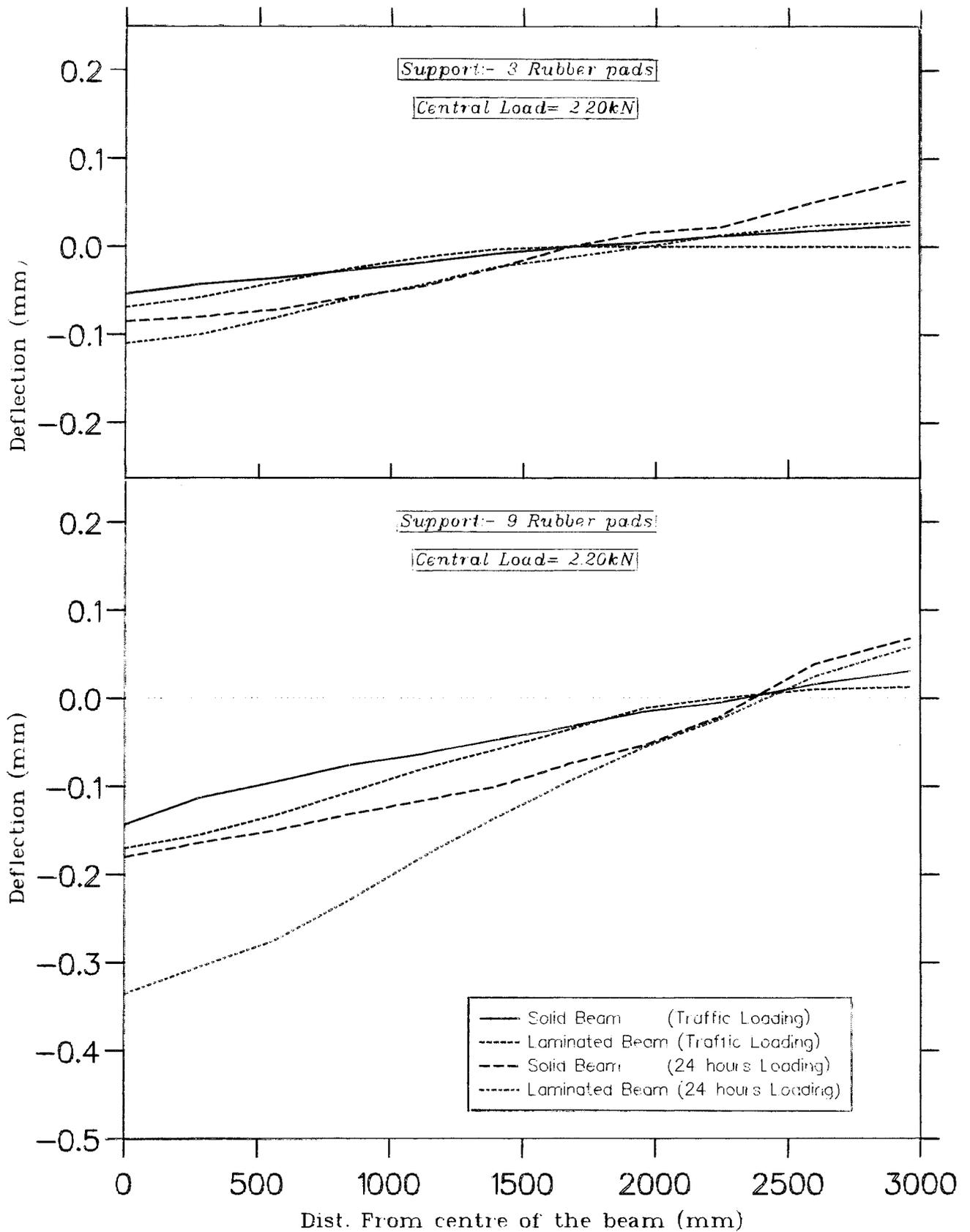
Fig 3 & 4 Deflected profiles of laminated and solid RC beams on an elastic subgrade with varying duration of load and subgrade stiffness. (Half section shown)
