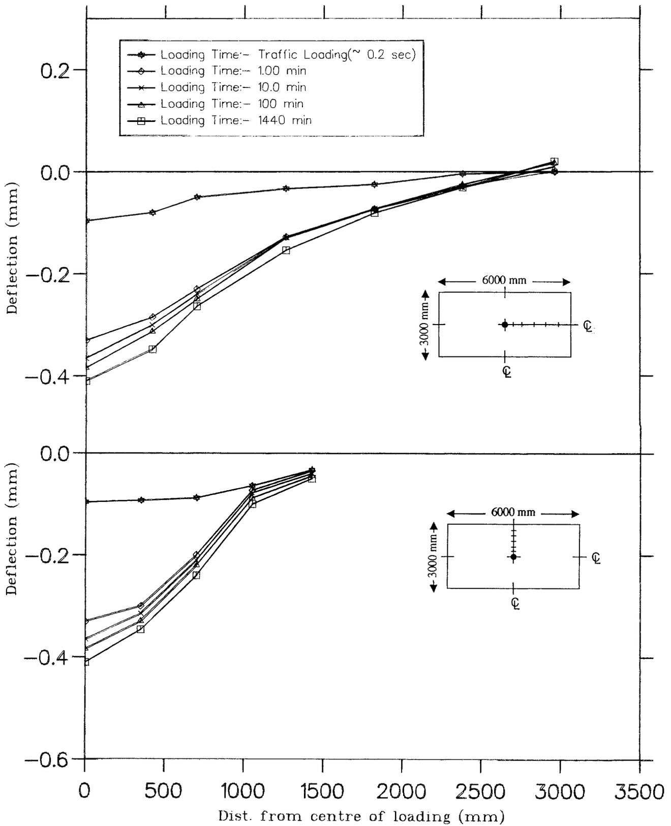
Fig 1 & 2 Deflected profile of laminated RC slab on an elastic subgrade with varying duration of 50 kN load. (Half section shown)
