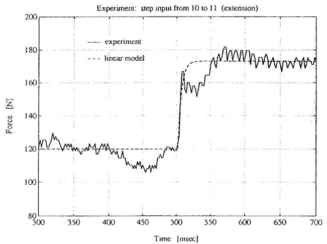
Fig.2 Step Input Response of the Semi-active Damper for Constant Suspension Velocity of 0.18 m/sec and its Linear Approximation
