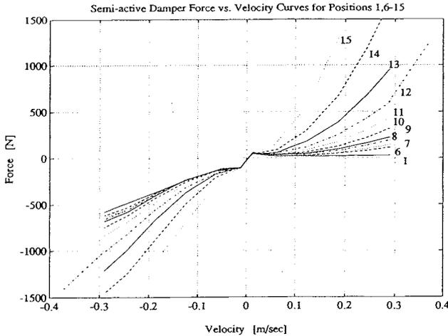
Fig.6 Semi-active Damper force vs. Velocity Curves
