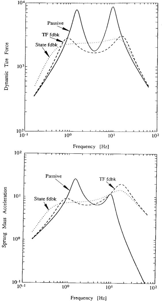
Fig.4 Frequency Responses of Quarter Car Model (A Comparison between State Feedback and Tire Force Feedback Cases)
