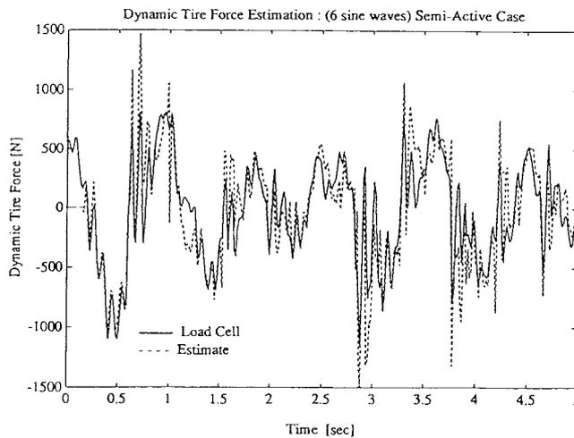
Fig. 9 Comparison of Measured and Estimated Dynamic Tire Force (sum of six sine wave input case)
