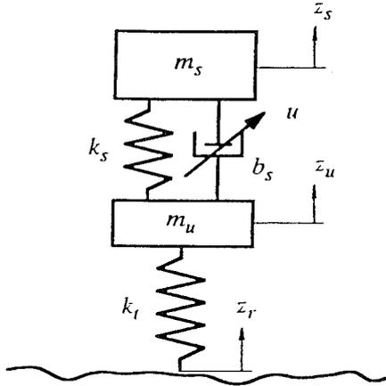
Fig.1 Quarter Car Semi-active Suspension Model
