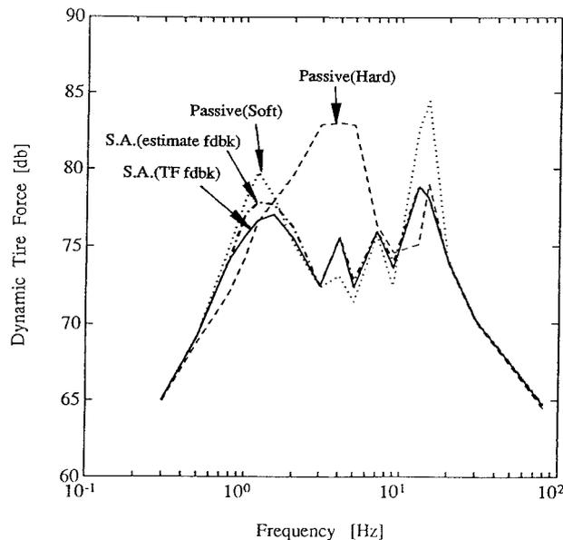
Fig. 10 Comparison of Frequency Responses of Passive and semi-active suspensions
