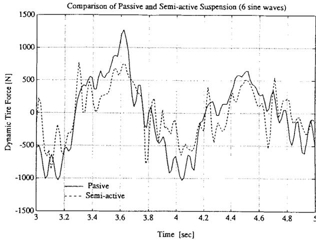
Fig. 8 Comparison of Dynamic Tire Force for Sum of Six Sine Waves Road Input Case
