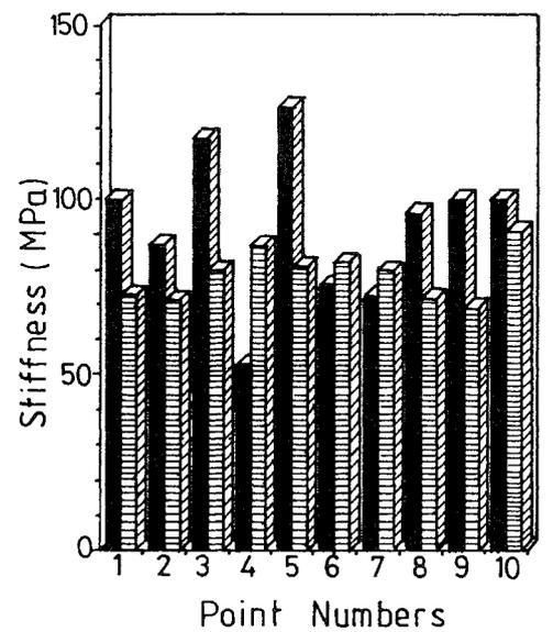
Fig. 2 Changes in Pavement Moduli due to Reinstatement
