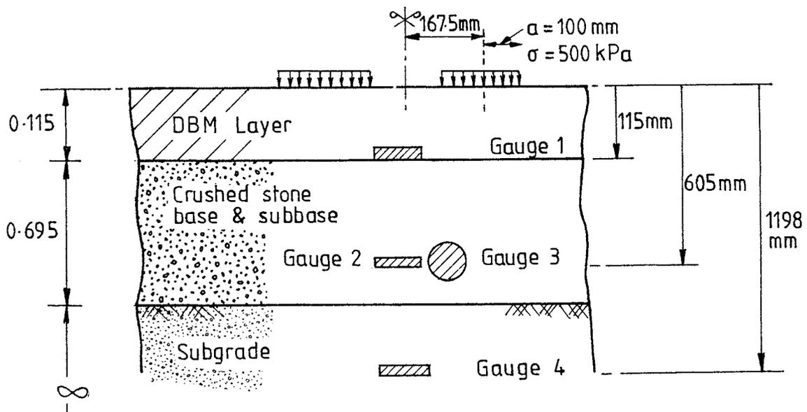
Fig. 3 Stress measurements under Heavy Vehicle
