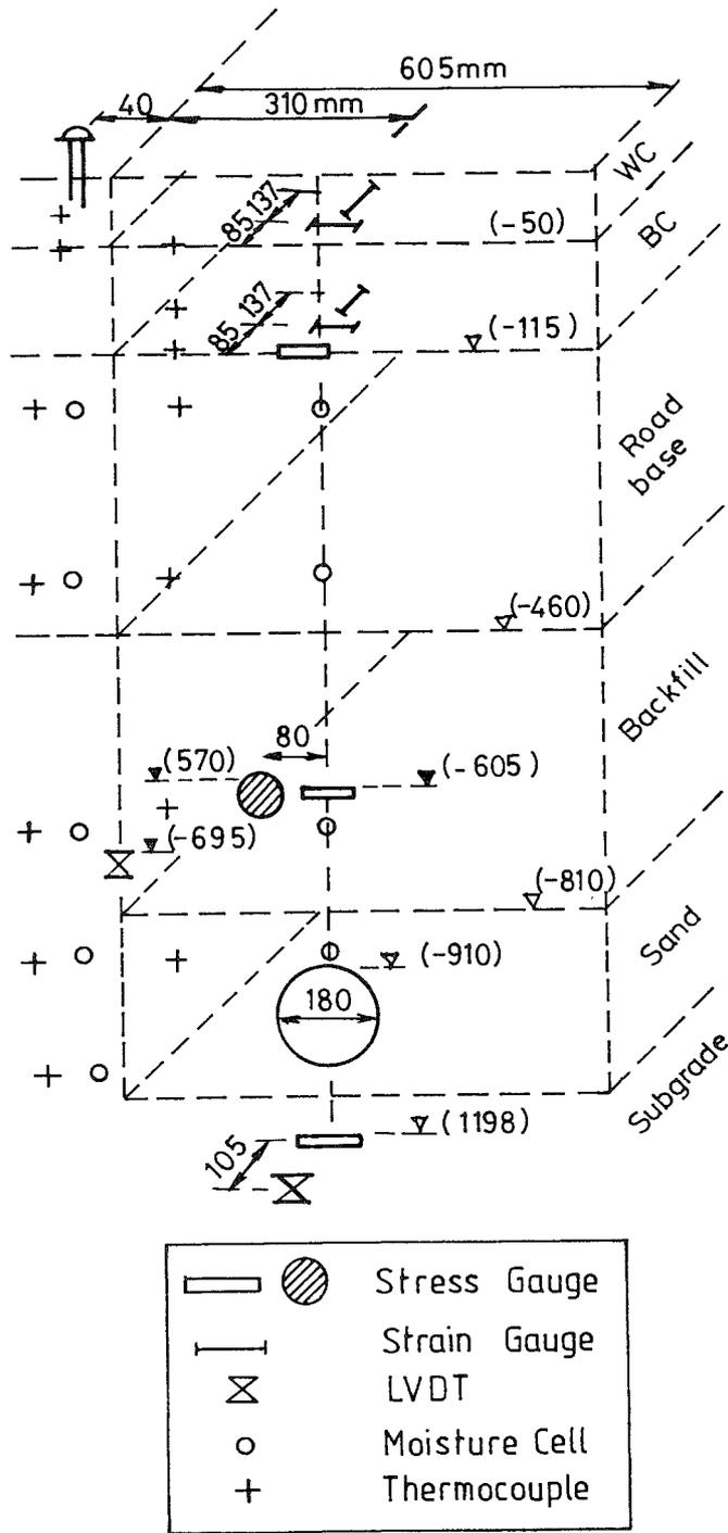
Fig. 1 Cross-section of the Test Road at QUB site showing instrumentation.
