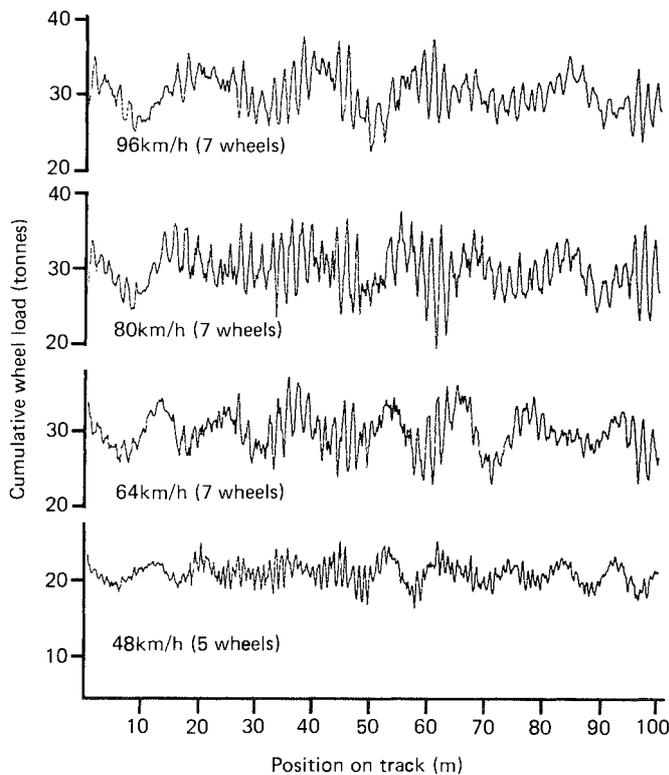
Fig.4 Sum of the loads under 5 or 7 wheels of air sprung semi-trailer bogies on the TRL track (rough section)
