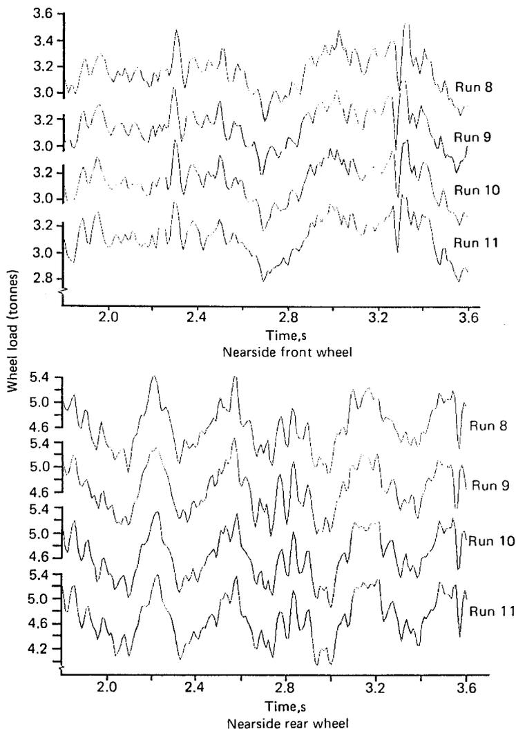
Fig.1 Dynamic wheel loads for a 2 axle HGV at 80 km/h on a trunk road
