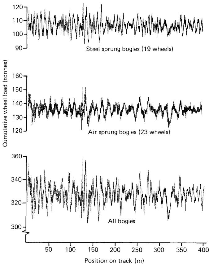
Fig.6 Sum of the loads under all the wheels of air and steel sprung semi-trailer bogies at speeds of 32 to 96km/h on the TRL track (medium section)
