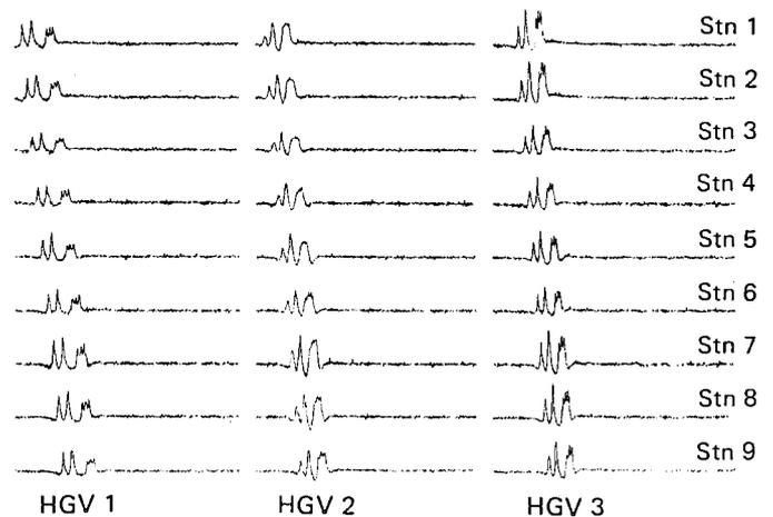
Fig. 7 Pavement strains at 9 stations on a motorway under the nearside wheels of 3 5 axle HGV
