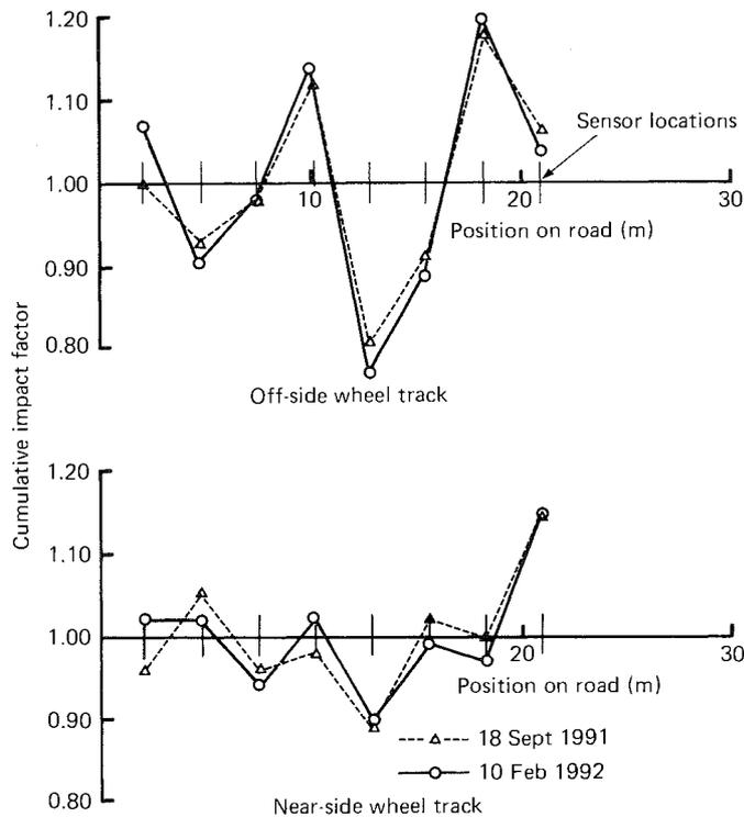
Fig.8 Cumulative impact factor for heavy vehicle wheels on a trunk road
