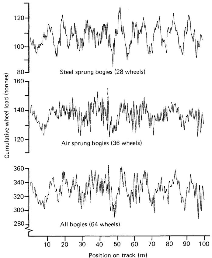
Fig.5 Sum of the loads under all the wheels of air and steel sprung semi-trailer bogies at speeds of 32 to 96km/h on the TRL track (rough section)
