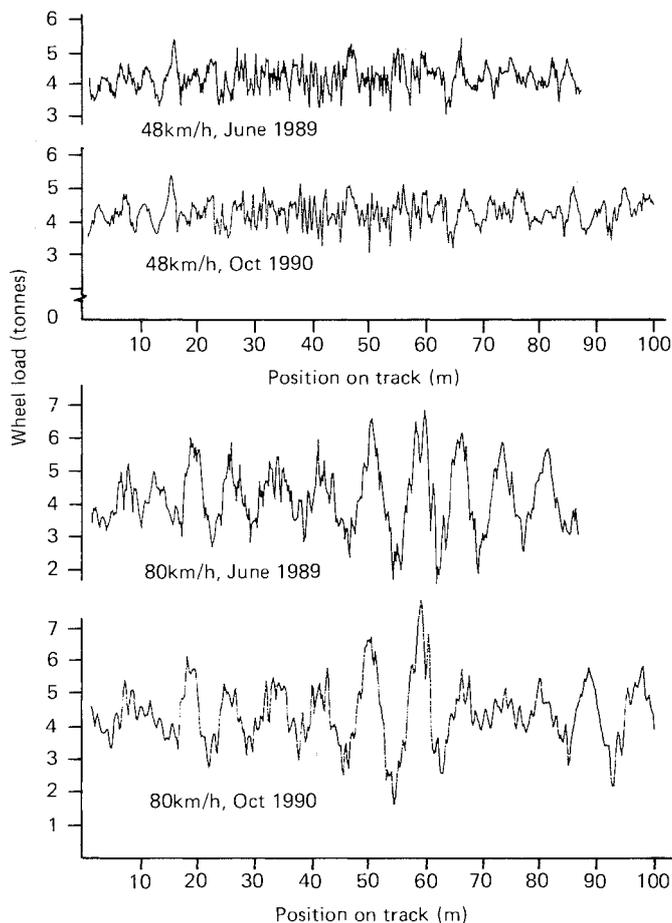
Fig.2 Dynamic loads for one wheel of a semi-trailer bogie on the TRL track (rough section)
