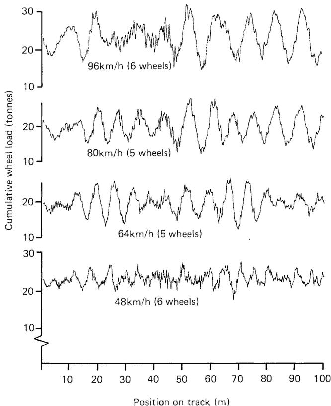
Fig.3 Sum of the loads under 5 or 6 wheels of steel sprung semi-trailer bogies on the TRL track (rough section)
