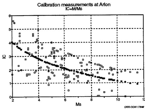
Fig. 6. Measured values of impact factor  $I_c$  against axle load
