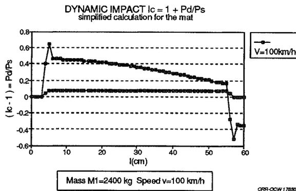
Fig. 7. Impact effect of the capacitive mat assessed from a theoretical vehicle model
