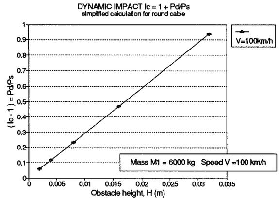
Fig. 1 Theoretical effect of obstacle height on  $I_c$
