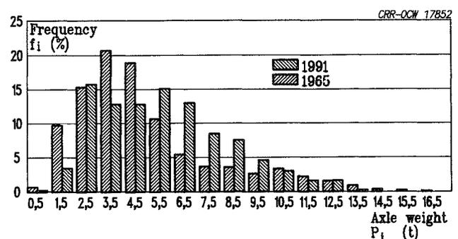
Fig. 9 Developments in the load spectrum on Belgian roads between 1965 and 1991
