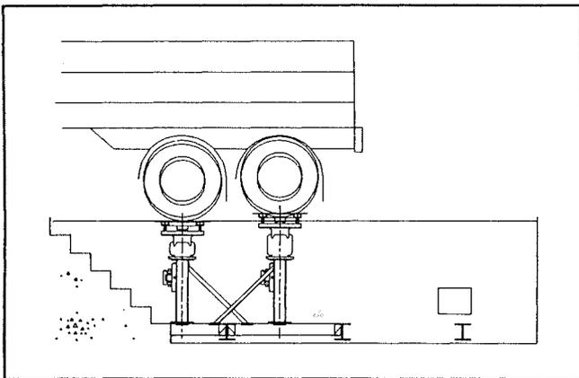
Figure 1. Vehicle support for shaker rig.
