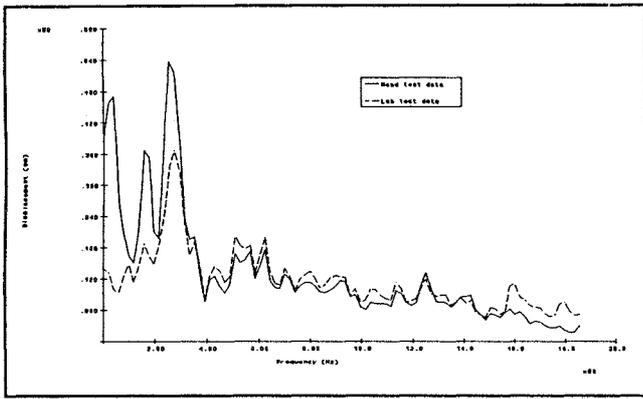
Figure 7 Spectral distribution of rear suspension deflections.
