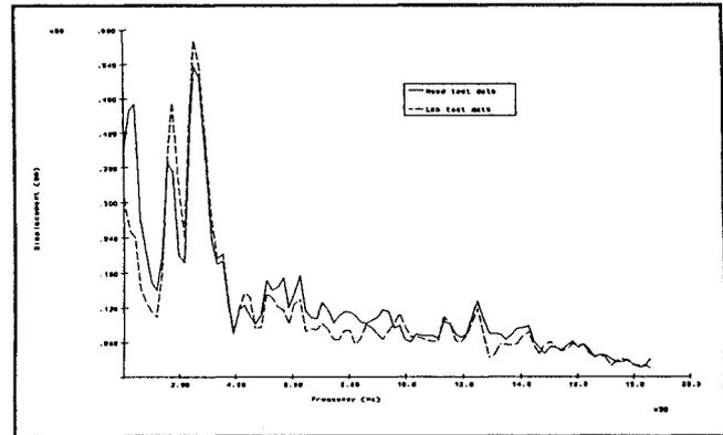
Figure 5 Spectral distribution of rear suspension deflections
