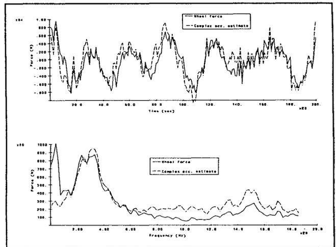
Figure 2. Wheel force by complex accelerometer method.
