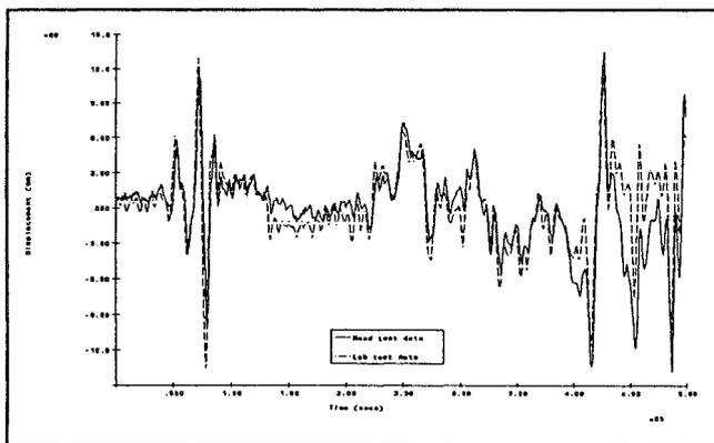
Figure 8 Suspension deflection signal for rear wheel
