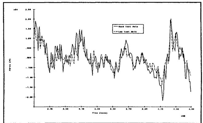
Figure 10 Force signal for rear wheel.
