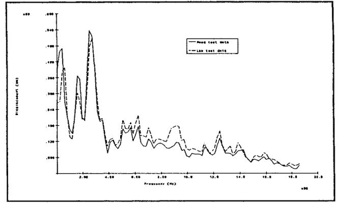
Figure 9 Spectral distribution of rear suspension deflections.
