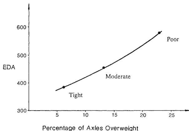
Fig 2. Damage effect of overloading
