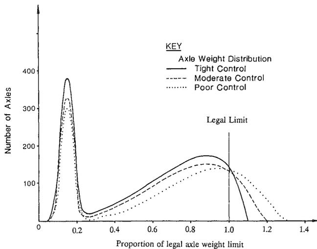
Fig 1. Axle weight distribution for varying compliance levels
