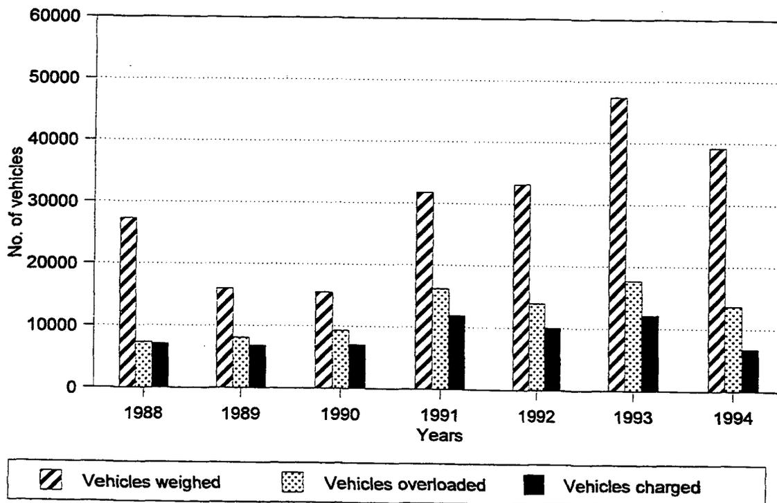
Figure 2. Vehicles weighed, overloaded and charged per year in KwaZulu-Natal: 1988 to 1994
