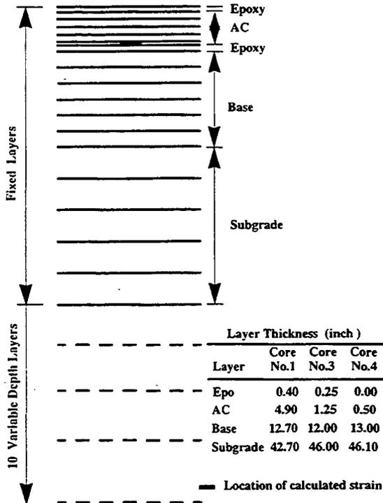
Figure 15. Pavement models used in SAPSI analysis
