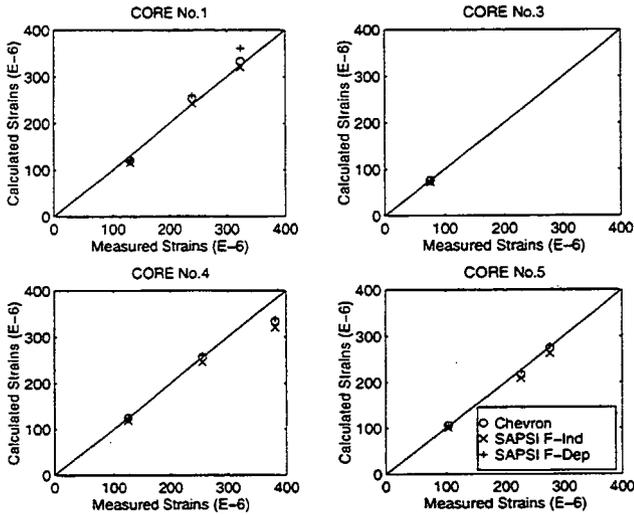
Figure 3. Predicted vs. measured strains-Oct.'91 FWD tests
