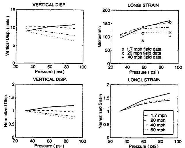
Figure 19. Effect of pressure on pavement response
