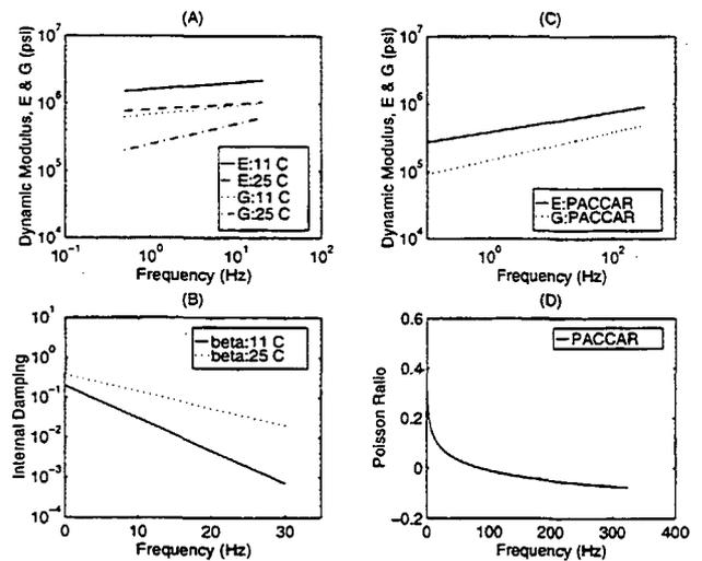
Figure 2. Asphalt concrete properties versus frequency
