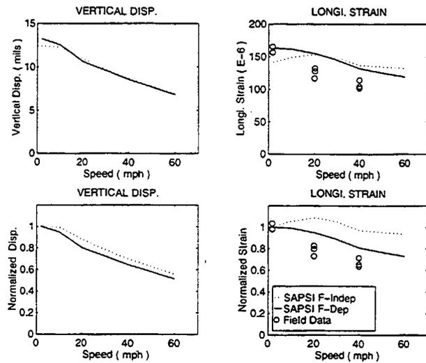
Figure 16. Effect of speed on pavement response - Core 1
