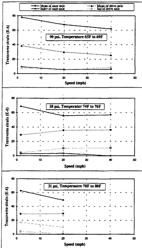
Figure 9. Transverse bottom strain in AC versus speed
