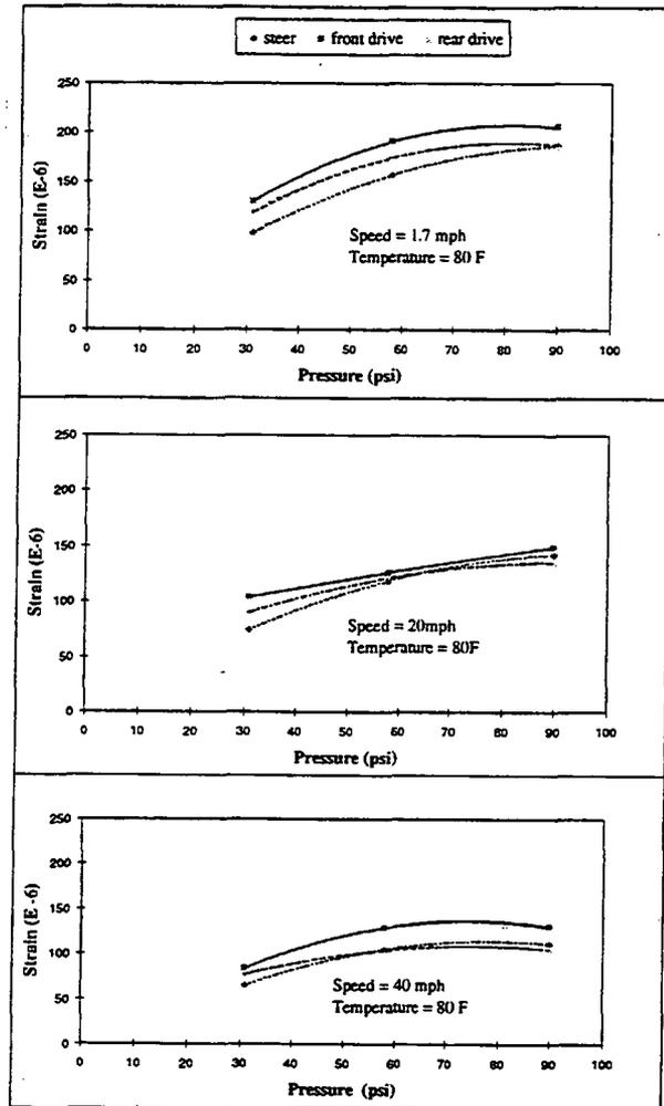
Figure 12. Bottom longitudinal strain in AC vs. pressure
