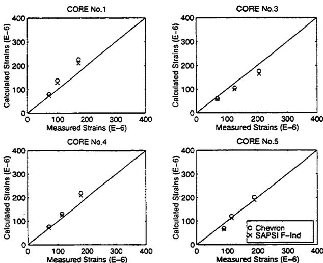
Figure 5. Predicted vs. measured strains-Feb.'93 FWD tests
