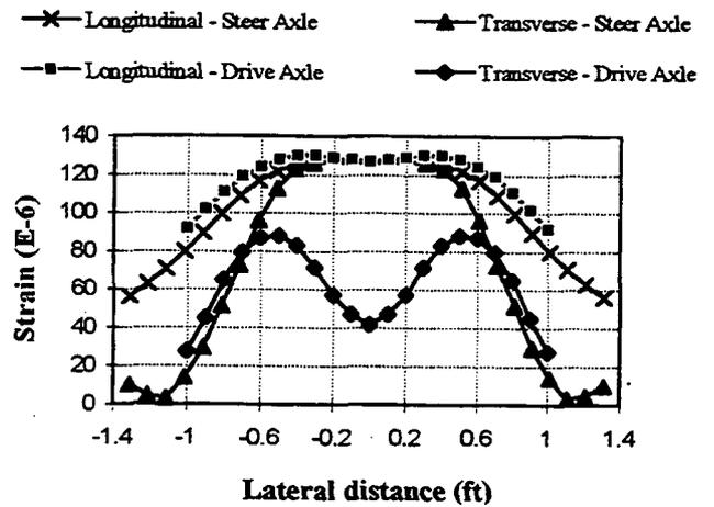
Figure 10. Typical lateral distributions of strain
