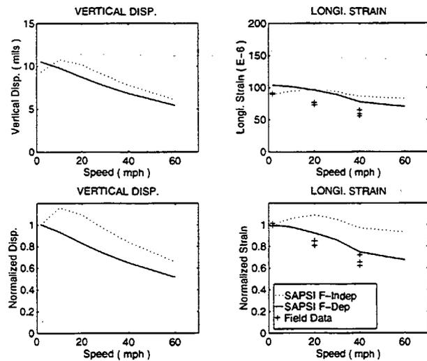
Figure 17. Effect of speed on pavement response - Core 3
