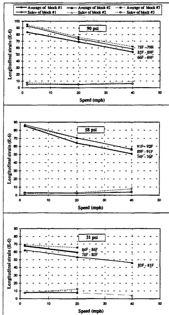
Figure 8 Longitudinal bottom strain in AC versus speed
