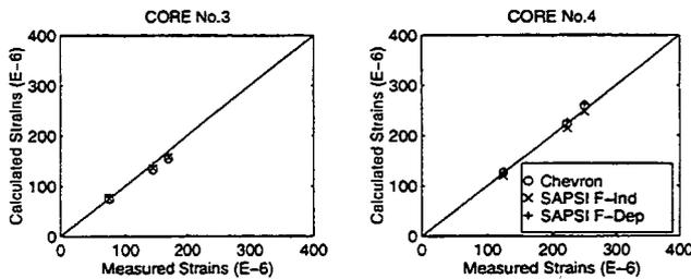
Figure 4. Predicted vs. measured strains-June'92 FWD tests
