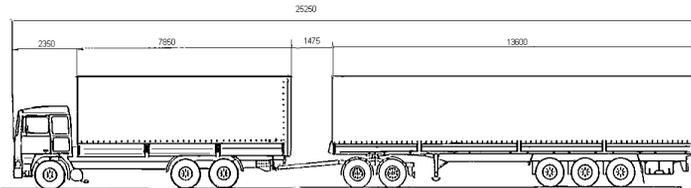
Figure 1: Vehicle A (truck, full-trailer)
