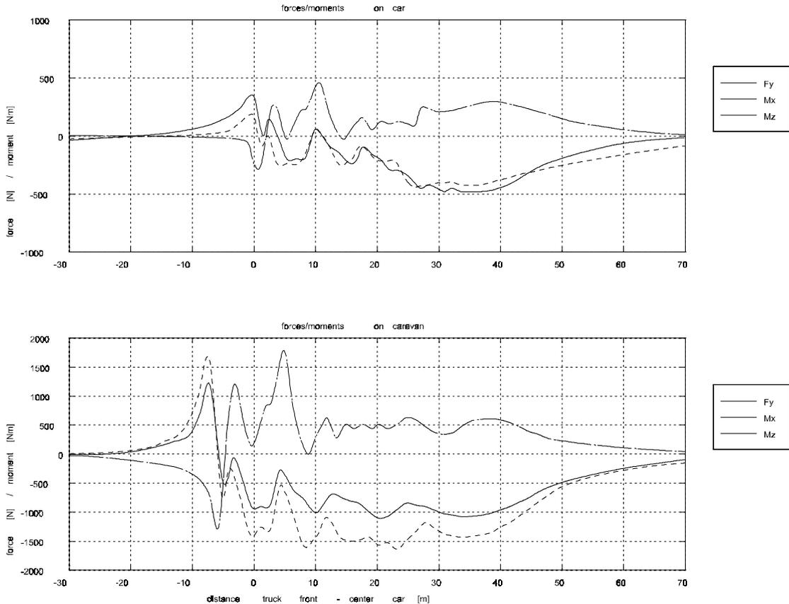
**Figure 10: Aerodynamic lateral force and yaw and roll moment on the passenger car and caravan**
