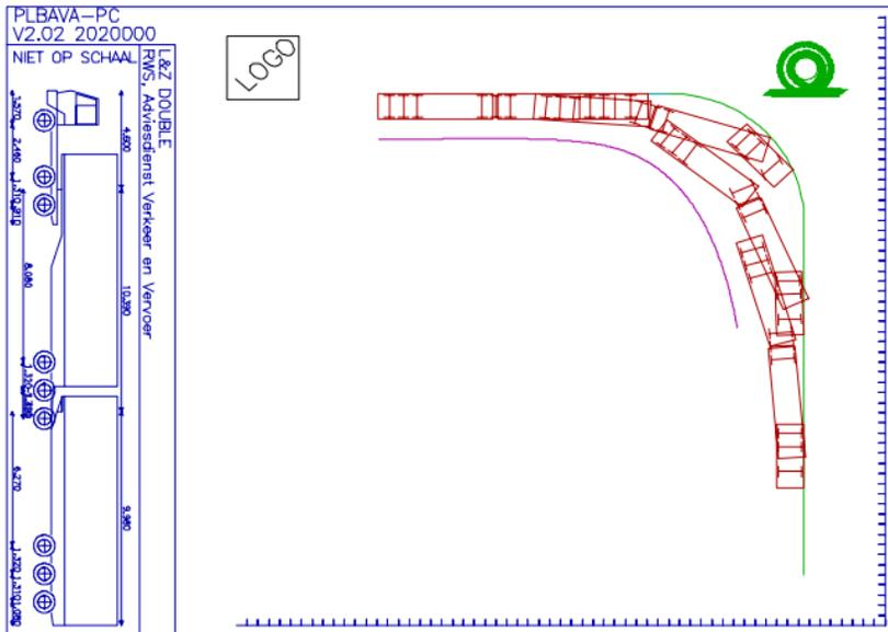
Figure 6: Swept path calculation (Vehicle C)
