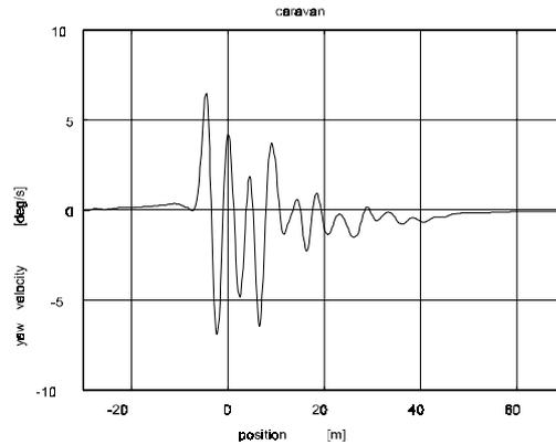
**Figure 11: Lateral acceleration and yaw velocity in COG of passenger car and caravan**
