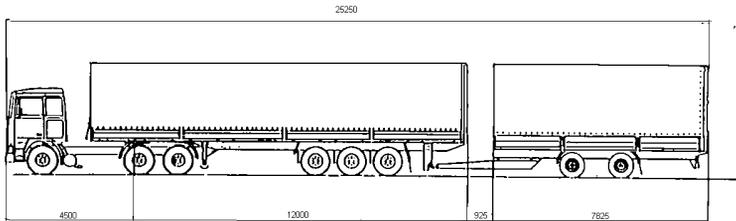
Figure 2: Vehicle B (tractor, semi-trailer, central axle trailer)
