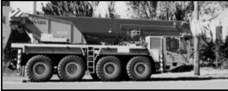
Figure 3 Demag AC205 Hydro-pneumatic Crane
