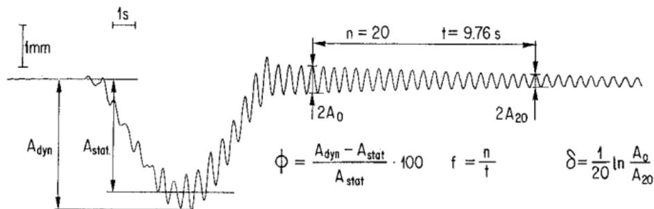
**Figure 16 Time history with the definitions of the dynamic increment  $\phi$  [%], the fundamental frequency  $f$  [Hz] and associated damping decrement  $\delta$  (or, in percent of critical:  $\xi = \delta/2\pi$ ). (from Cantieni, 1983)**
