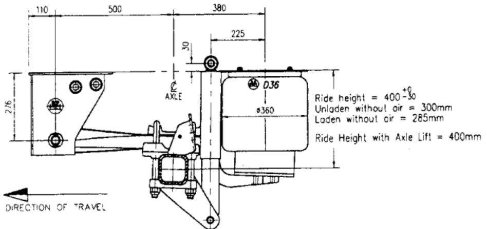
**Figure 1 Air suspension - BA trailer**
