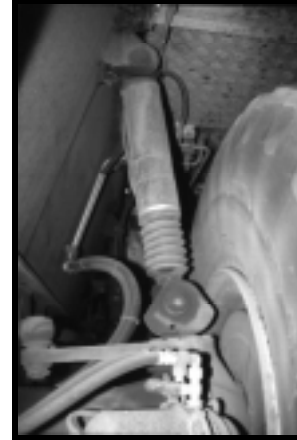
Figure 4 Hydro-pneumatic suspension of Demag AC205 Crane
