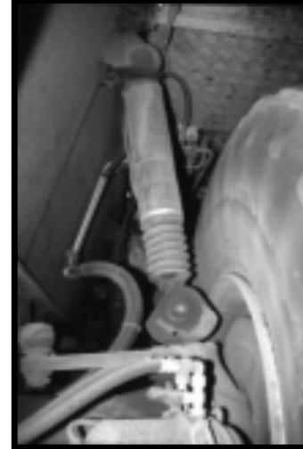
*Figure 4 Hydro-pneumatic suspension of Demag AC205 Crane*
