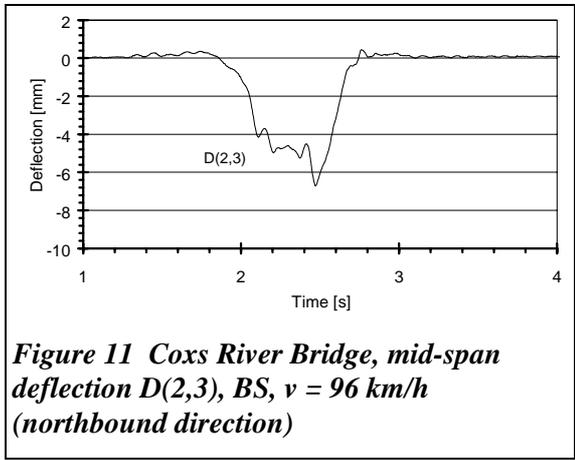
**Figure 11** Coxs River Bridge, mid-span deflection D(2,3), BS,  $v = 96$  km/h (northbound direction)
