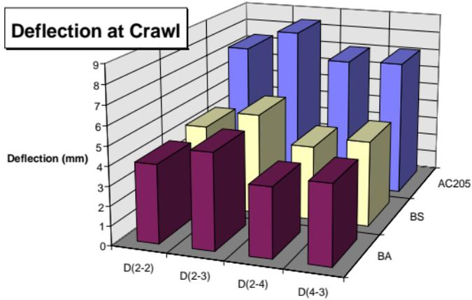
*Figure 12 Comparison of Deflections at Crawl Speed*
