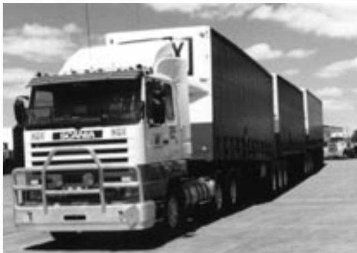
*Fig 3. A Typical B-Triple Combination operated in Queensland*
