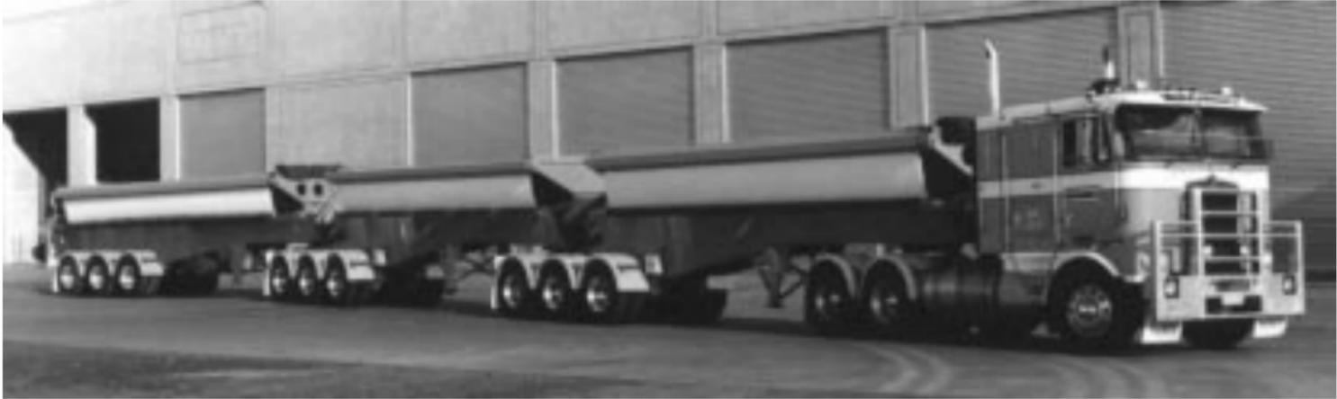
*Fig 1. A B-Triple Combination*
