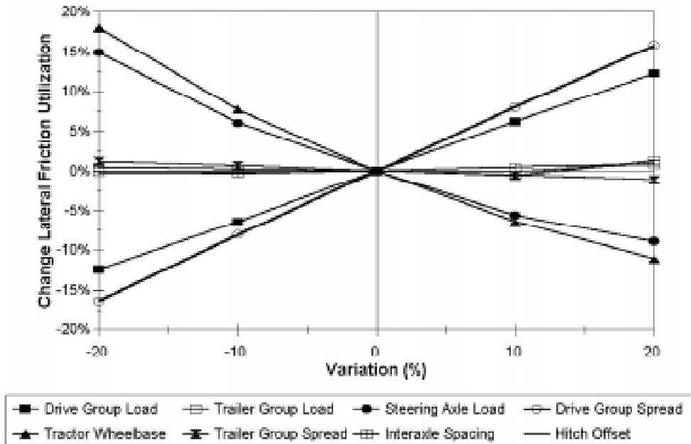
Figure 6 - Sensitivity of lateral friction utilization of steer tires to changes in various configuration parameters.
