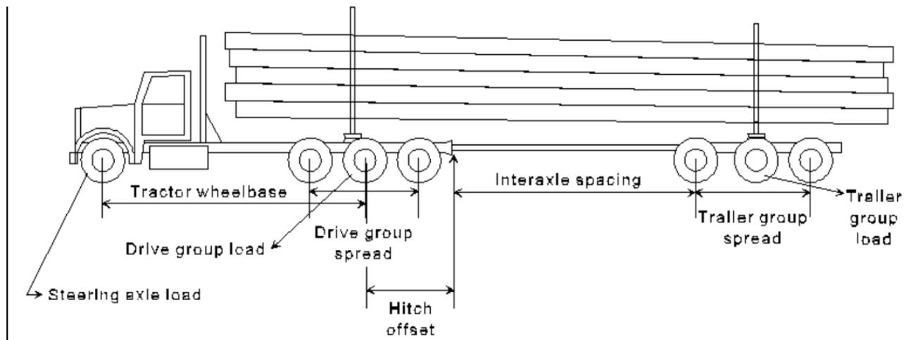
**Figure 5 - Tractor and trailer parameters.**
