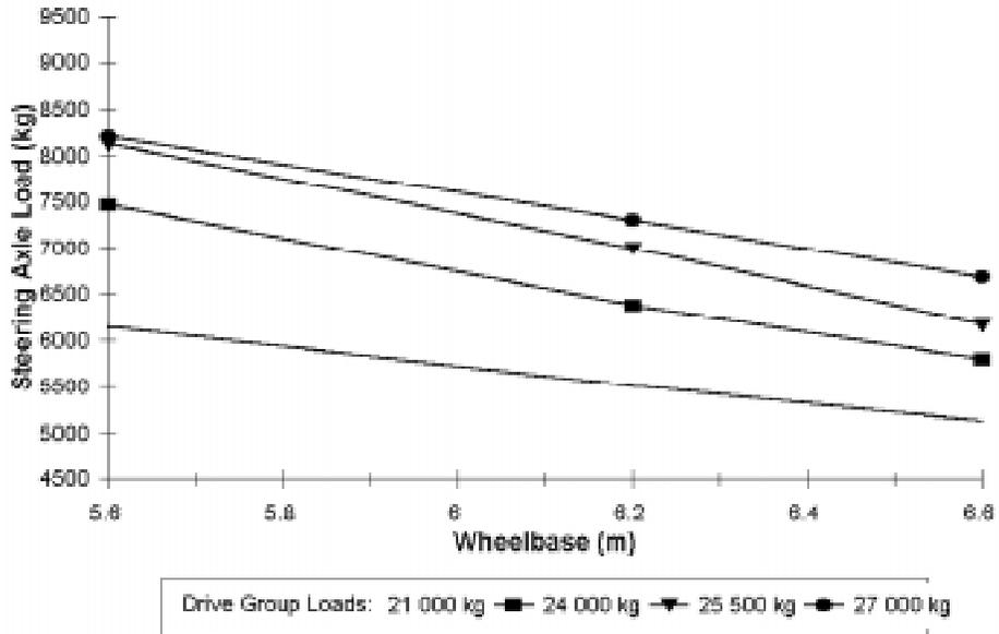
Note: Acceptable steering axle / load wheelbase combinations for each loading condition fall above the respective line. Lines define 80% LFU; LFU decreases (improved steering performance) above lines.
