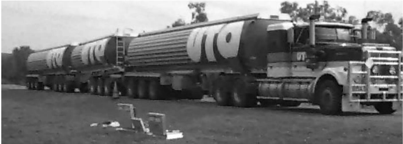
**Figure 20 Innovative vehicle AB-Triple**
