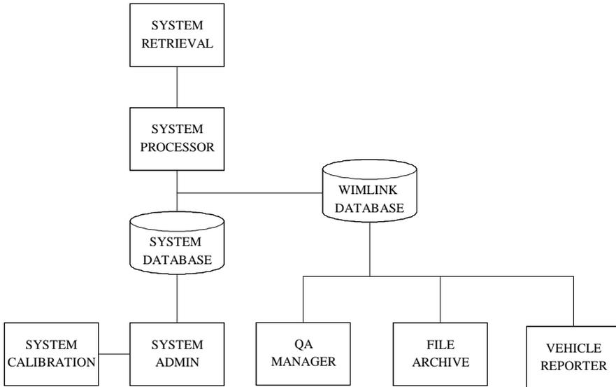
*Figure 2. Top Level Design of WIMLINK*
