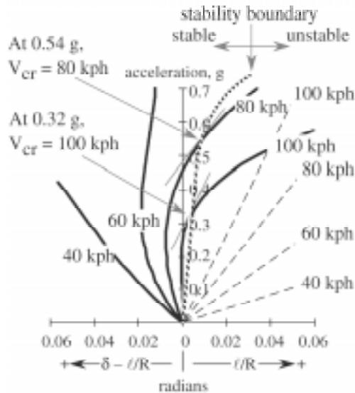
Fig. 4. Slopes of the V-handling curves indicate the critical velocities and the stability boundary for the complex vehicle
