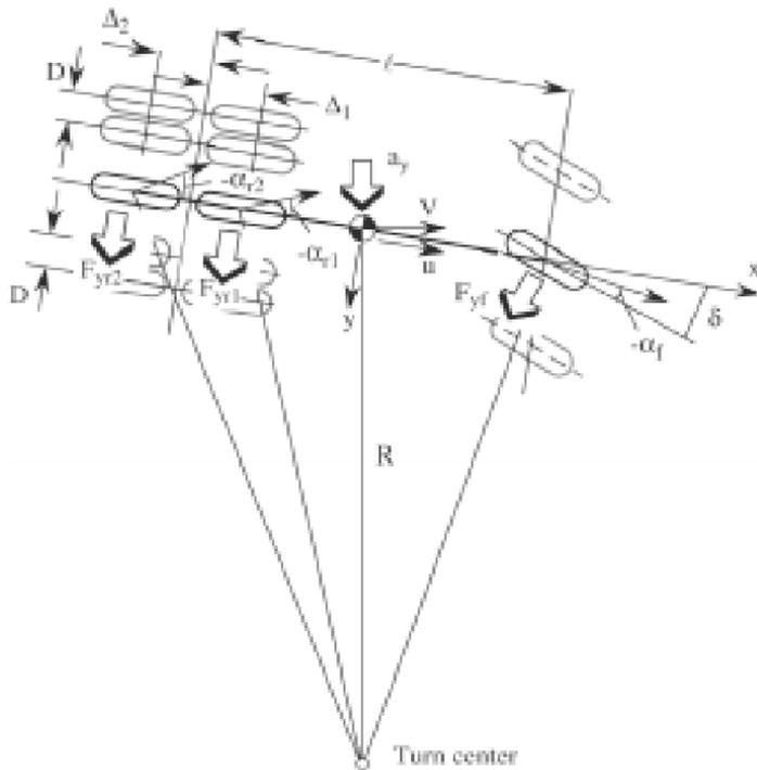
**Fig. 6. Simplified model of the three-axle truck in a steady turn**
