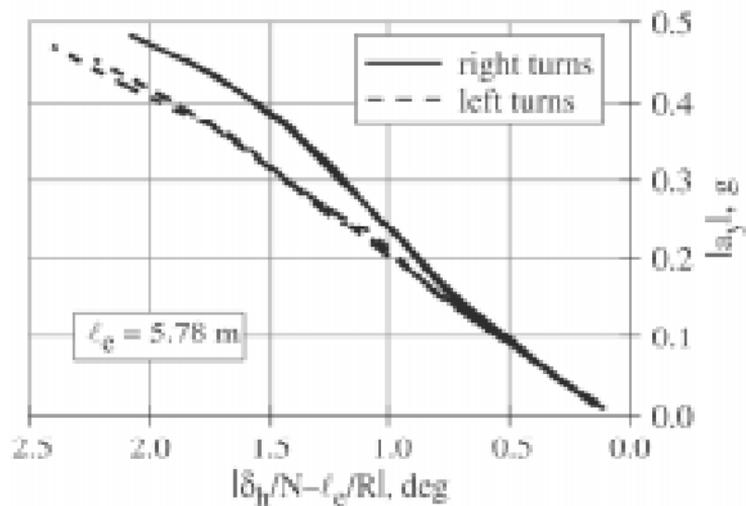
**Fig. 14. Handling diagram for all simulation results based on the equivalent wheelbase**
