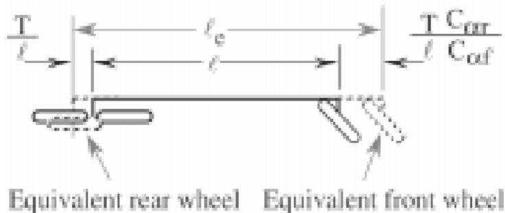
**Fig. 7. Physical interpretation of the equivalent wheelbase of a three-axle truck**
