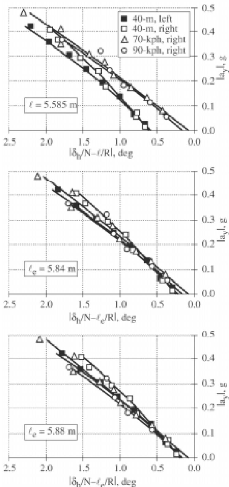
**Fig. 11. Handling diagrams derived from test-track data**
