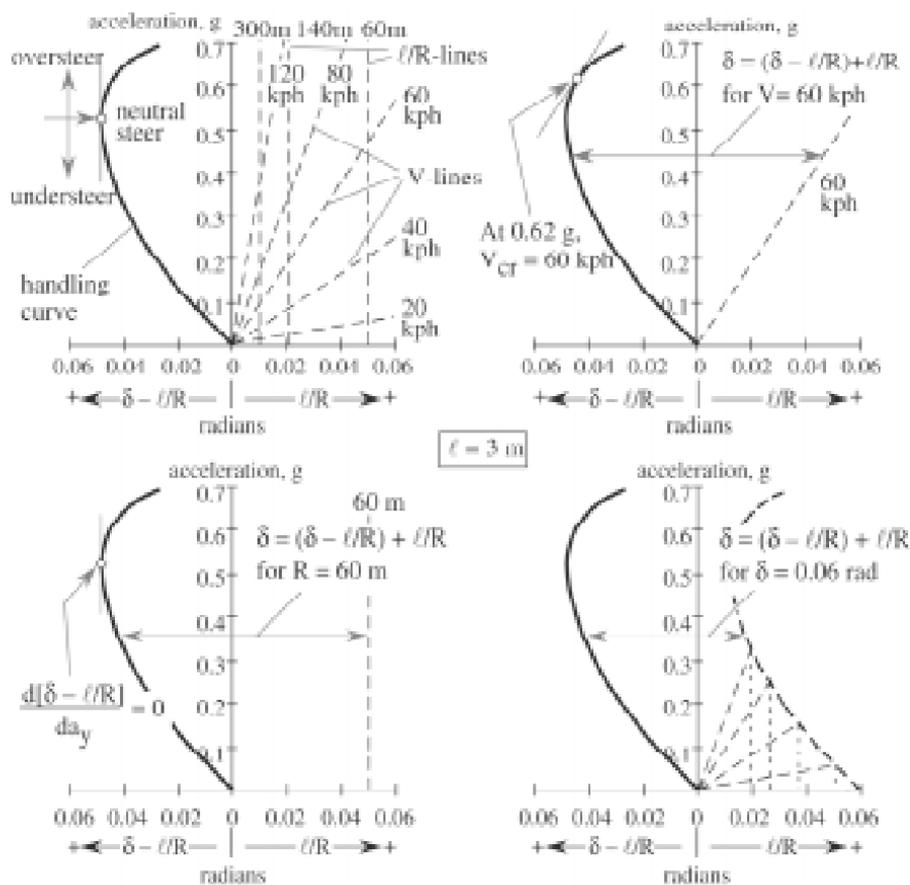
Fig. 2. Handling diagrams for a nonlinear, simple vehicle
