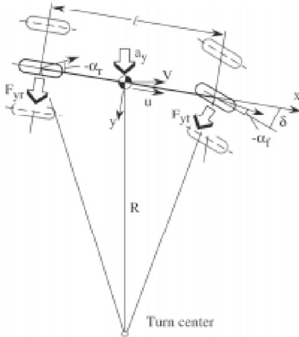
**Fig. 1. Simplified model of a simple vehicle in a steady turn**
