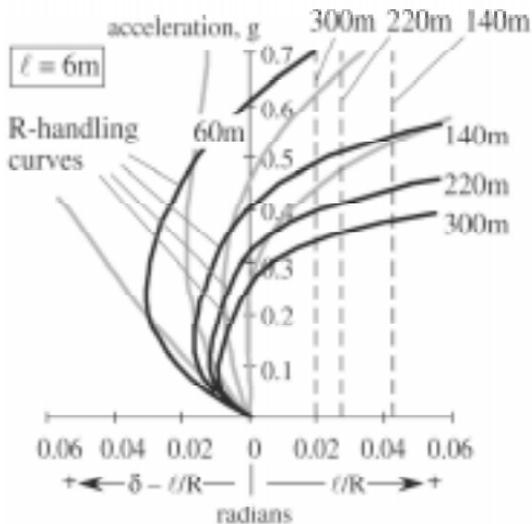
**Fig. 5. R-handling curves superimposed on the V-handling curves of a nonlinear, complex vehicle**
