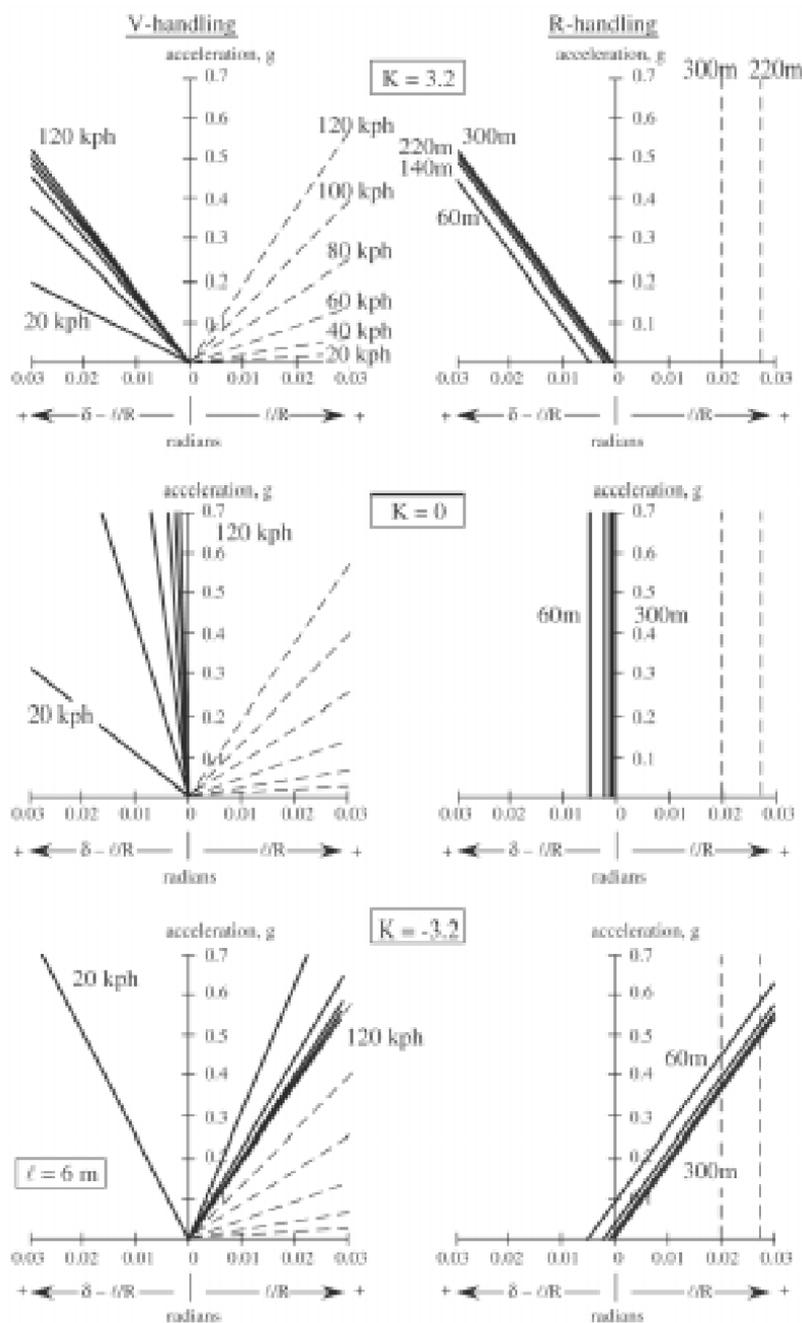
Fig. 8. Handling diagrams for a linear, three-axle truck
