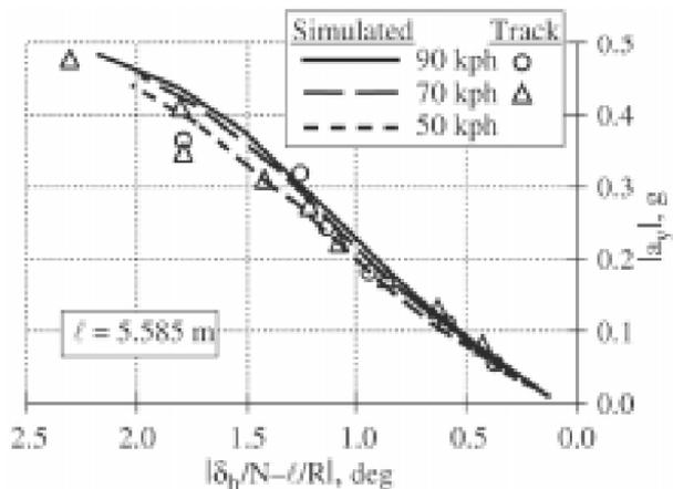
Fig. 12. Simulated and actual right-turning, constant-velocity tests
