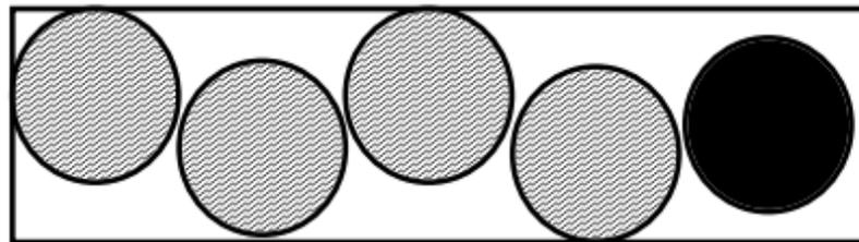
*Figure 11. Recommended loading pattern to achieve maximum stability.*
