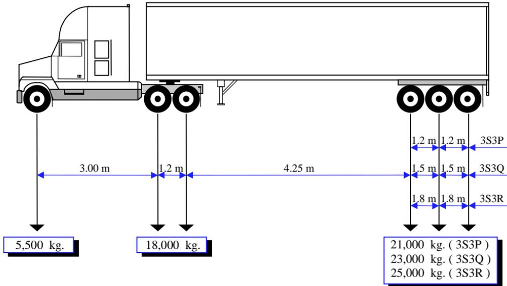
Figure 5 - Short Tridem Semi-Trailer Trucks ( 3S3P, 3S3Q, 3S3R )
