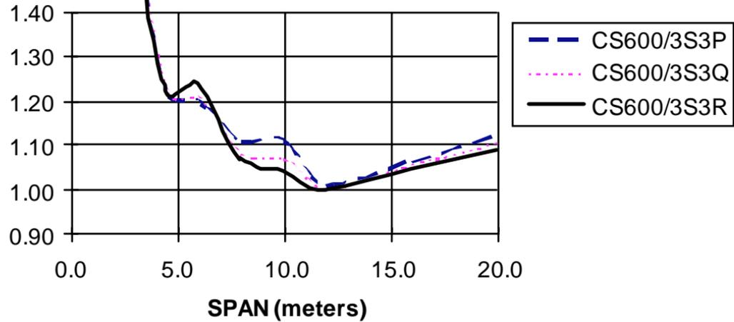
Figure 6 - Moment Comparison of Tridem Truck To CS600
