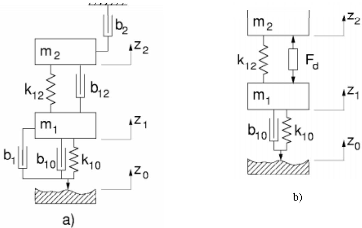
**Fig. 5 Combination of Sky-Hook, Ground-Hook and Passive Suspension**
