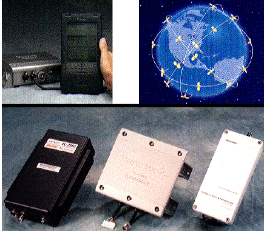
FIGURE 2: examples of typical transponders now available for LEO network (courtesy of ORBCOMM)s
