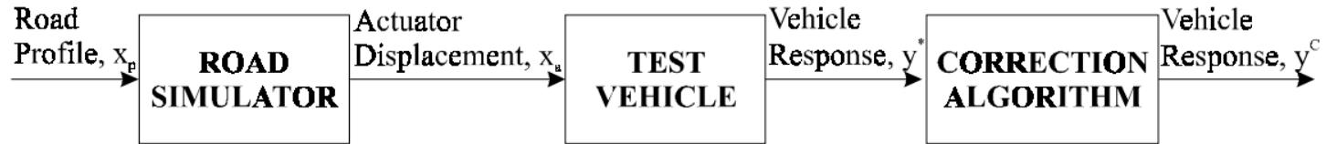
Figure 5. Block diagram of output correction system.
