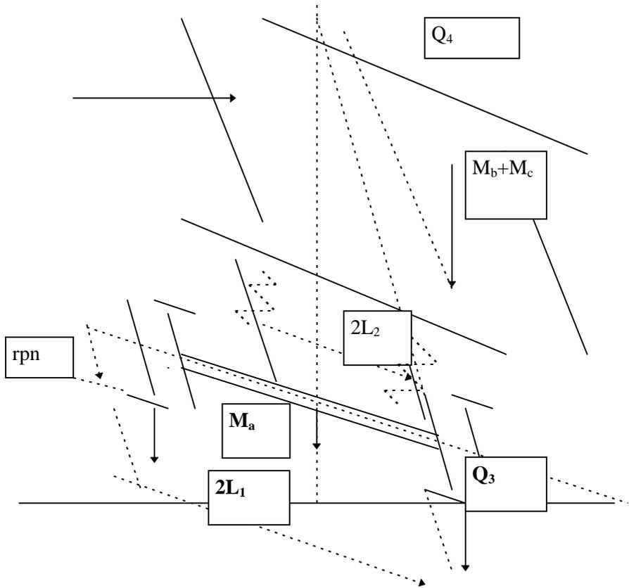
Figure 2: Dump truck model with leaf spring suspensions.
