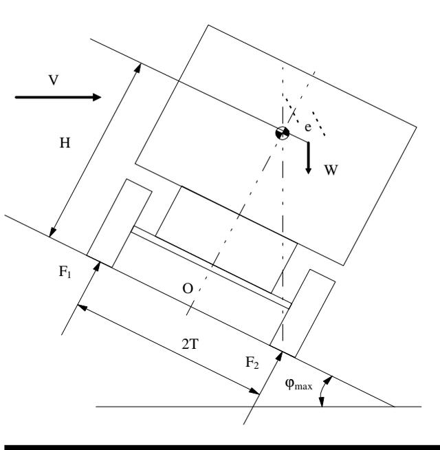
Figure 1: Vehicle model prior to roll-over with deflated suspensions
