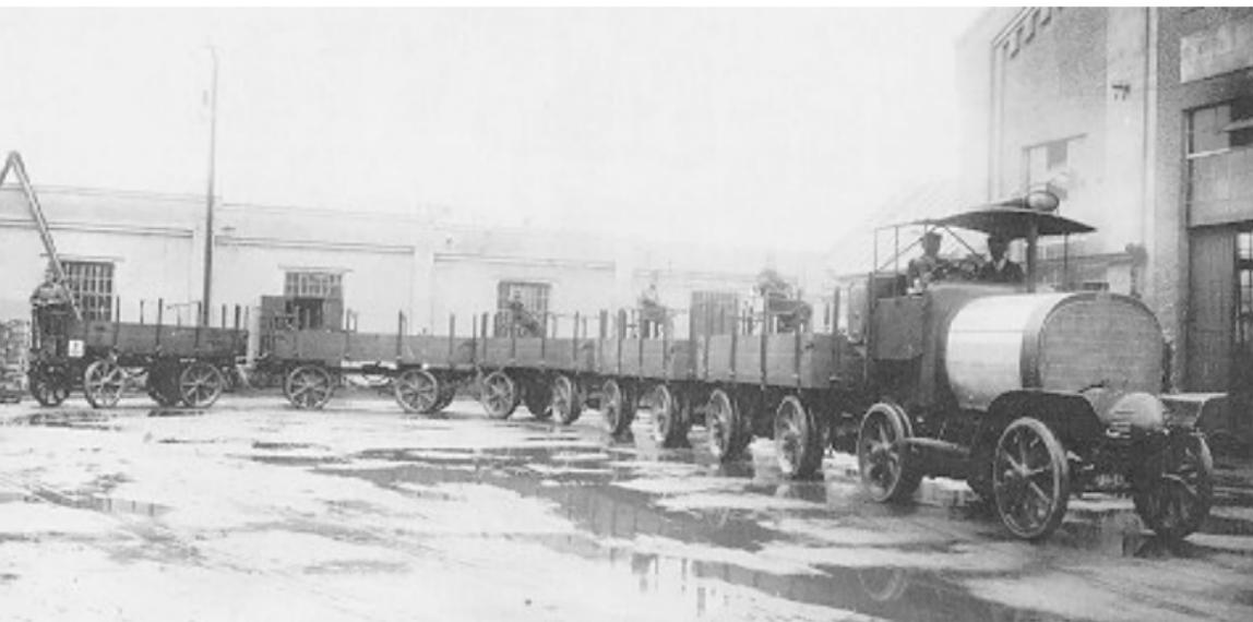
*Figure 1. Five-trailer all wheel steering vehicle (1911).*
