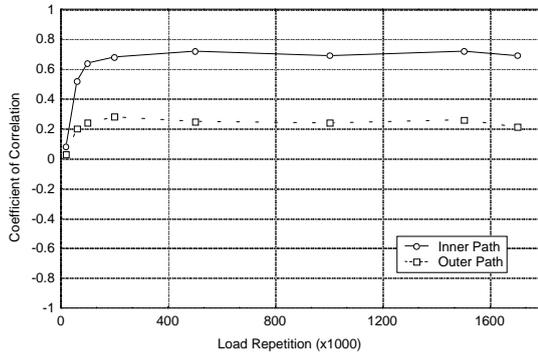
Figure 1 Cross Correlation between FWD Surface Deflection at 20k and VSD (Inner: ALL Data, Outer: SELECT Data)
