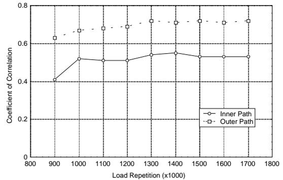
Figure 2. Correlation between FWD Deflection at 20k and Total Linear Cracking (SELECT Data)
