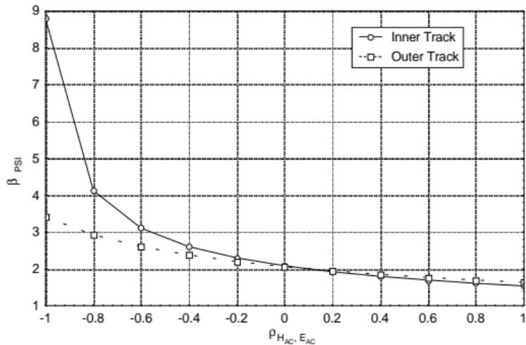
Figure 6. Effect of Correlation between  $H_{AC}$  and  $E_{AC}$  on Reliability Index
