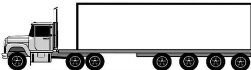
7-axle Tractor Semitrailer (3-S1111)
