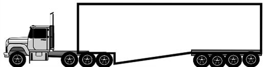
8-axle Tractor Semitrailer (4-S4)
