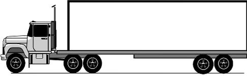
5-axle Tractor Semitrailer (3-S2)- "Van"
