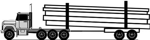
6-axle Tractor Semitrailer (4-S3)
