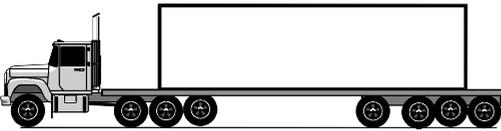
8-axle Tractor Semitrailer (4-S4)
