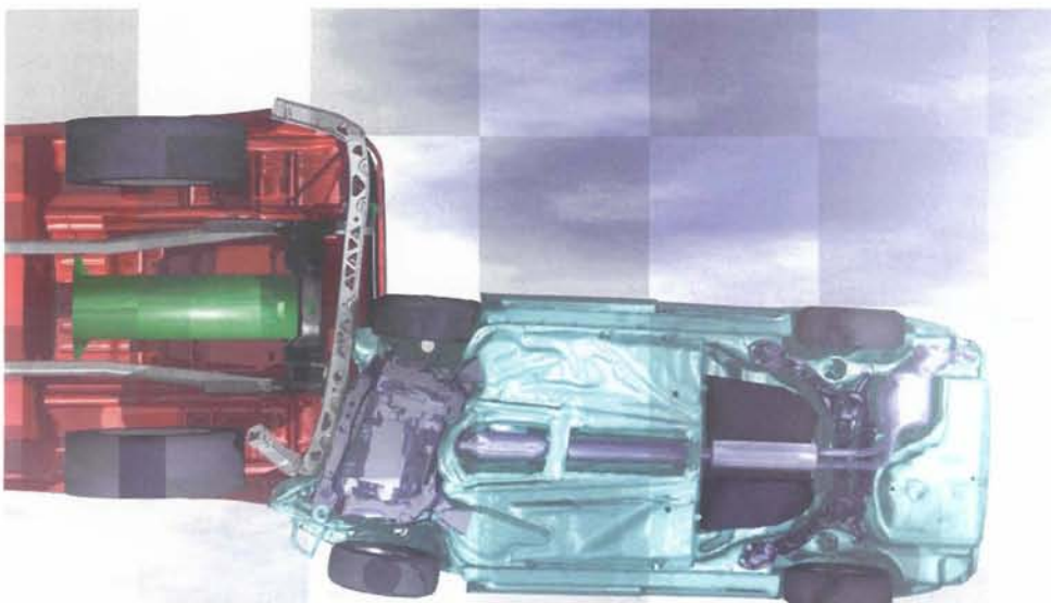
Figure 2 – Euro-NCAP type of impact set up. The figure shows maximum deformation of the car in the crash. Crash FE simulation from below.
