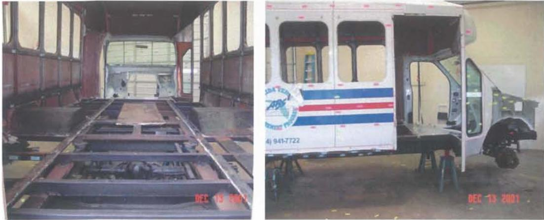
Figure 8. Disassembled Ford Eldorado Aerotech 240 transit bus.
