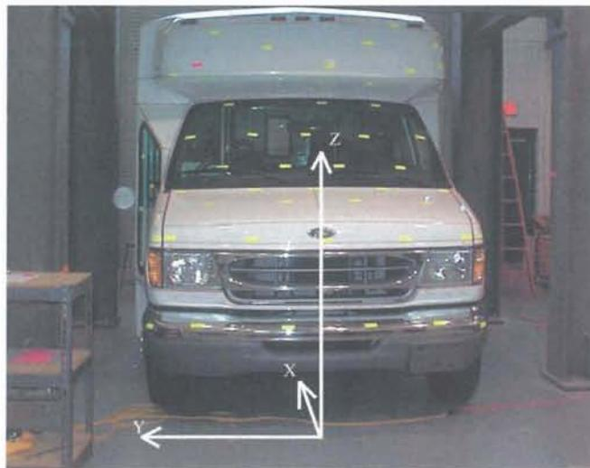
Figure 6 – User Coordinate System established for Eldorado Aerotech transit bus.
