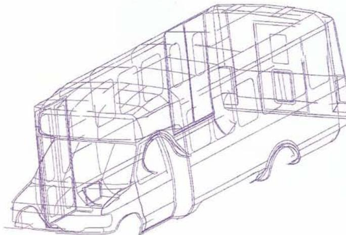
Figure 9. Polylines scanned for exterior bus components.
