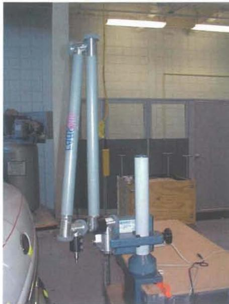
Figure 1 – Portable digitizing device: FARO Arm
