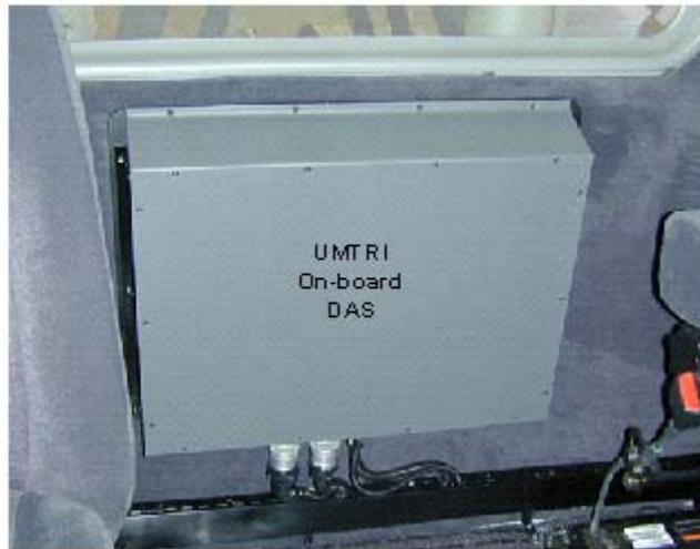
Figure 4. Installed UMTRI on-board data acquisition system.
