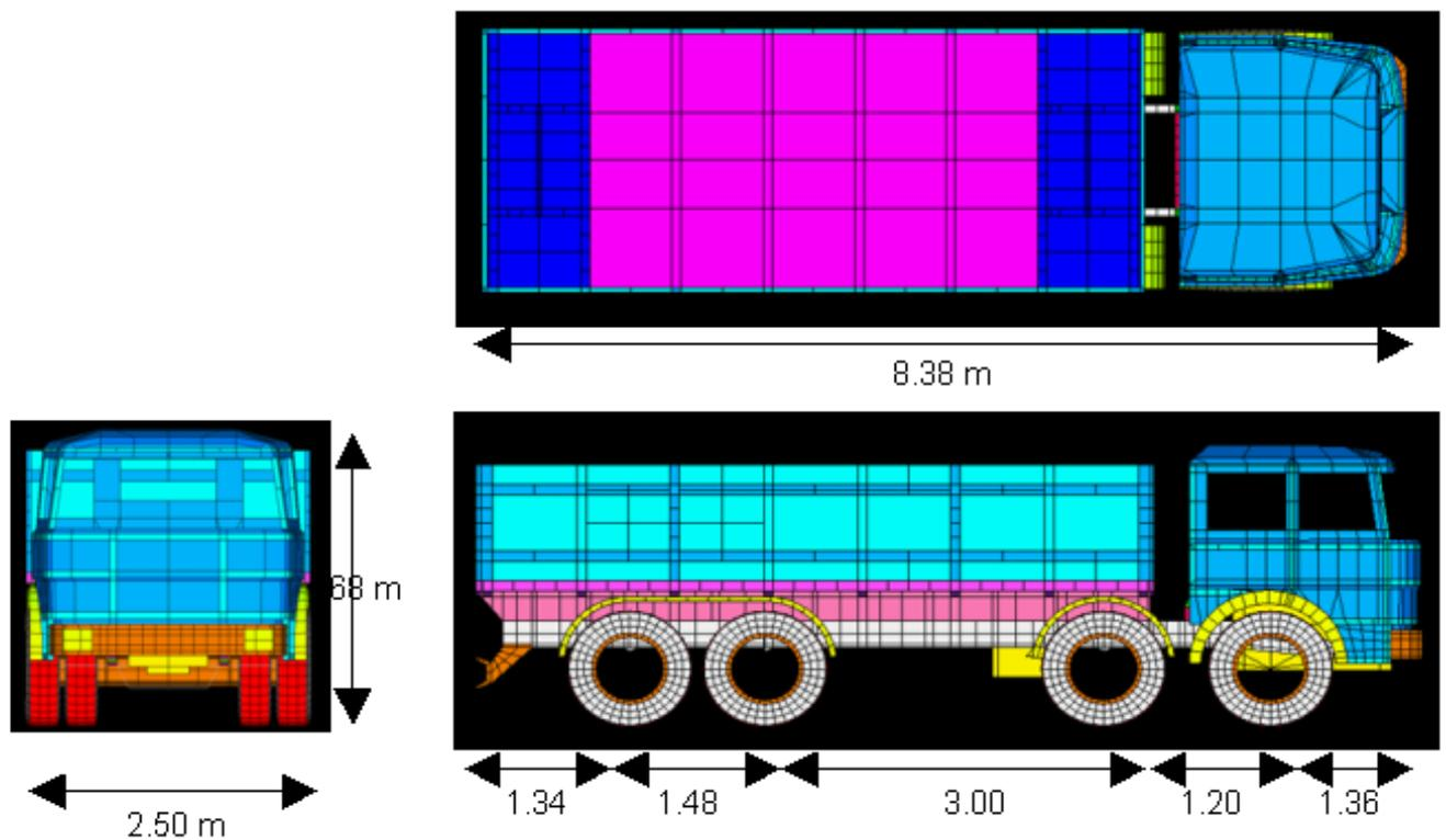
Figure 2. Finite element model of the heavy vehicle.
