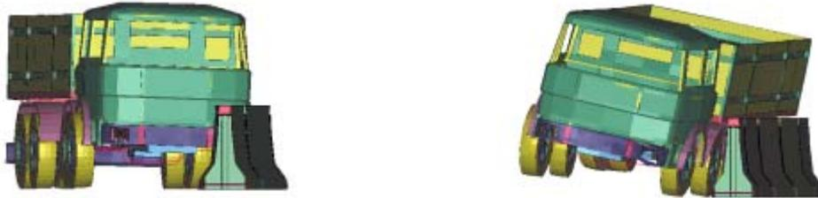
Figure 10. Shots from the simulation of HGV to reinforced concrete barrier impact.
