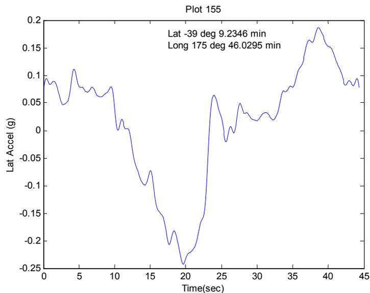
Figure 1. Lateral acceleration versus time for a curve on SH1.
