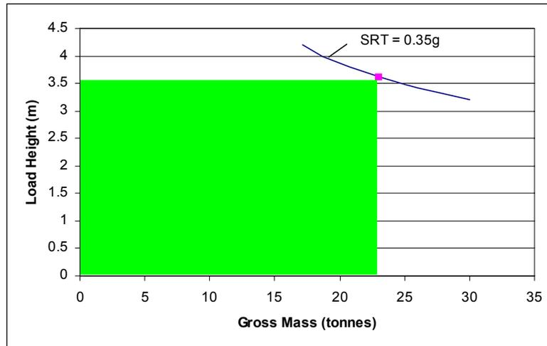
Figure 2. Height and weight to meet 0.35g SRT.
