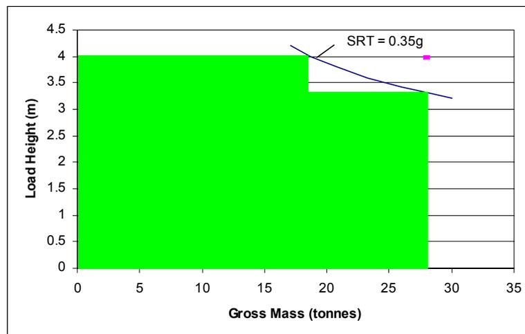
Figure 1. Reduced weight and height to meet 0.35g SRT.
