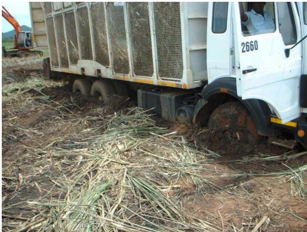
Figure 4. Infield damage caused by standard tyres.
