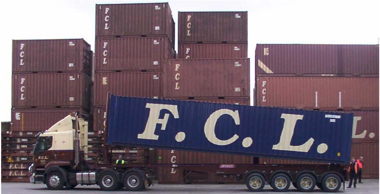
Figure 3. 40' intermodal container (35 t) in 50 t quad axle tipping combination.
