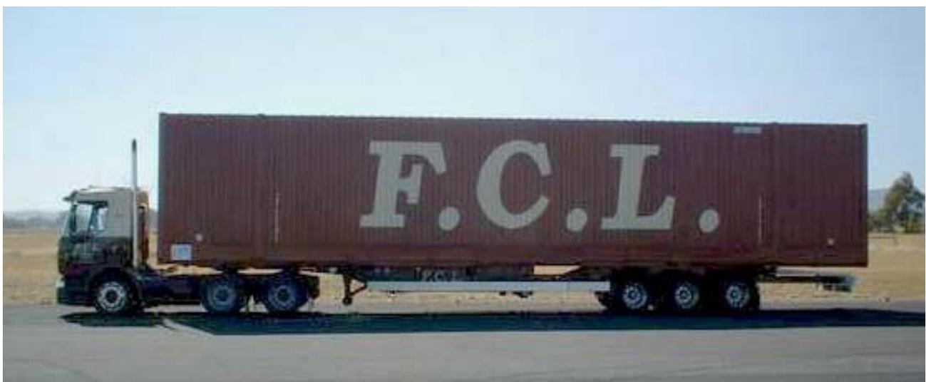
Figure 1. 54'6" intermodal container in 19 m tractor-semi-trailer combination.
