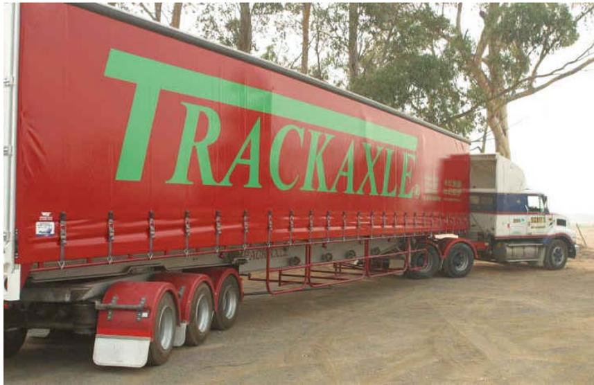
Figure 2. 52' trailer featuring "Trackaxle®" pivotal bogie system.
