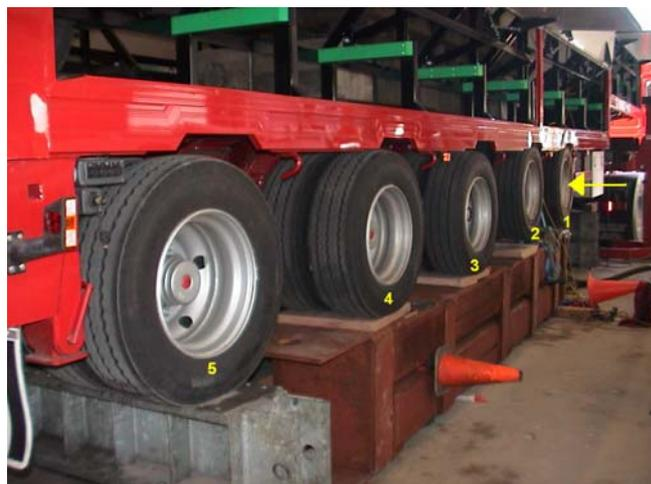
Figure 8. Levelled semi-trailer in the Lab for calibrating the measurement system.
