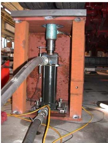
Figure 7. Hydraulic cylinders underneath the first axle.
