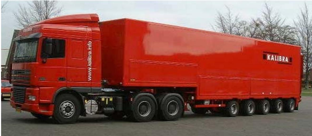
Figure 1. DAF 95XF530 (6x4) tractor and five axle Nootboom semi-trailer for calibration.
