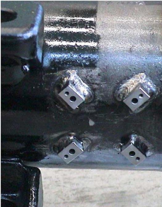
Figure 4. Mounting points for the set on the axle.
