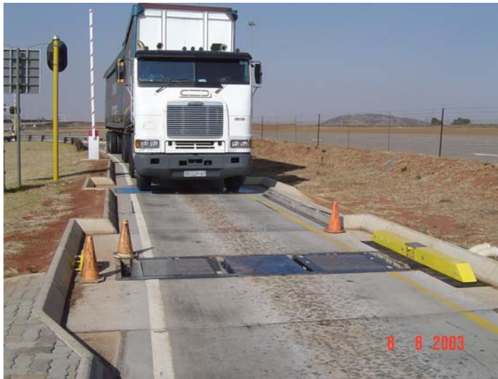
Figure 3. Quad (full) SIM pad configuration at a typical weighbridge site on National Road 3 (N3), near Heidelberg in Gauteng.
