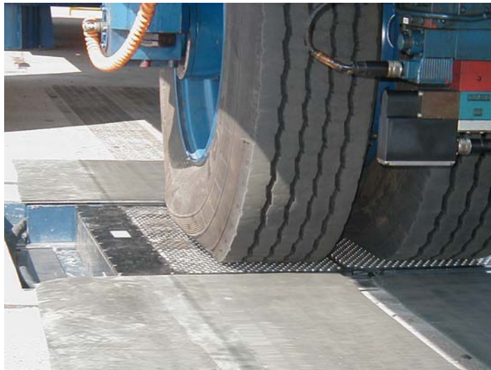
Figure 2. Twin (or dual) SIM pad configuration (used under Heavy Vehicle Simulator (HVS) with dual test tyres).
