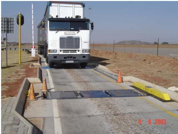
Figure 3. Quad (full) SIM pad configuration at a typical weighbridge site on National Road 3 (N3), near Heidelberg in Gauteng.
